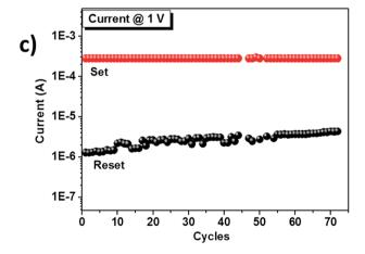
Fig. 10 (a) Cyclic I-V measured in the Au/PAG-IL/ITO system. (b) Zoom on the set and reset process in logarithmic scale. (c) Pulse characterization – sample was made to read at 1 V, by setting and resetting the device at -5 V and 2 V for  $500~\mu s$ .
