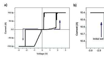
Fig. 4 (a) Initial cyclic I-V measured in the Au/PAG-IL/Au system. (b) Zoom on the initial set process taking place at -2.2 V.
