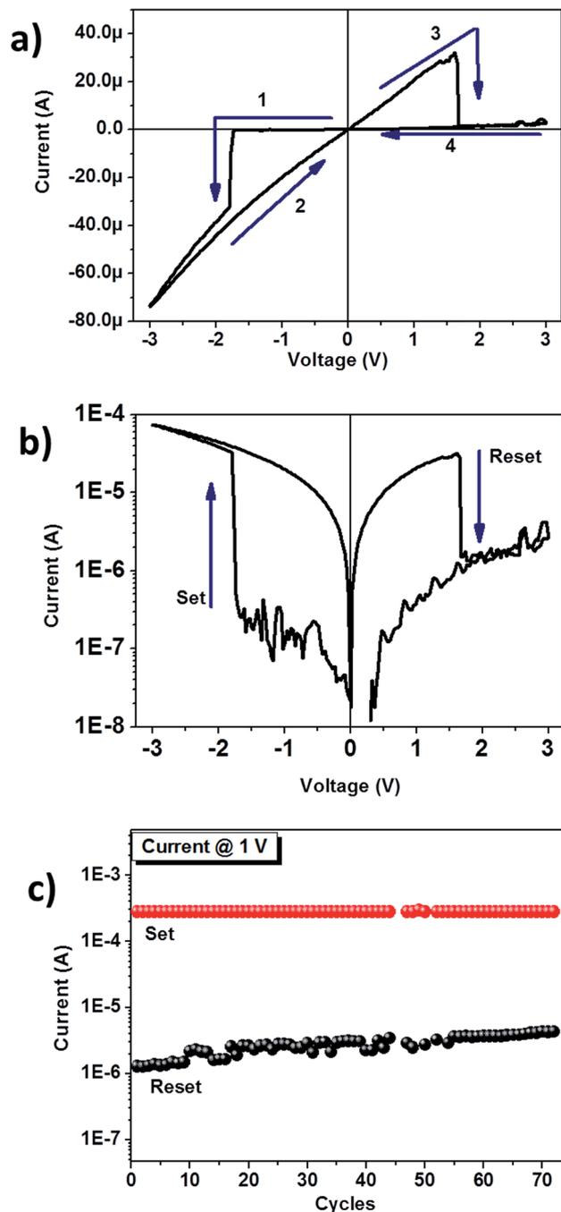
Fig. 10 (a) Cyclic  $I$ - $V$  measured in the Au/PAG-IL/ITO system. (b) Zoom on the set and reset process in logarithmic scale. (c) Pulse characterization – sample was made to read at  $1$  V, by setting and resetting the device at  $-5$  V and  $2$  V for  $500$   $\mu$ s.
