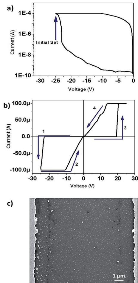
Fig. 3 (a) Initial set process, taking place at  $-25$  V. (b) Cyclic  $I$ - $V$  measured in the Au/PAG/Au system (c) FESEM image of the device with active switching matrix ( $\text{AgNO}_3$  and PVDF-HFP) spin coated between the gold electrodes, after electrical characterization.
