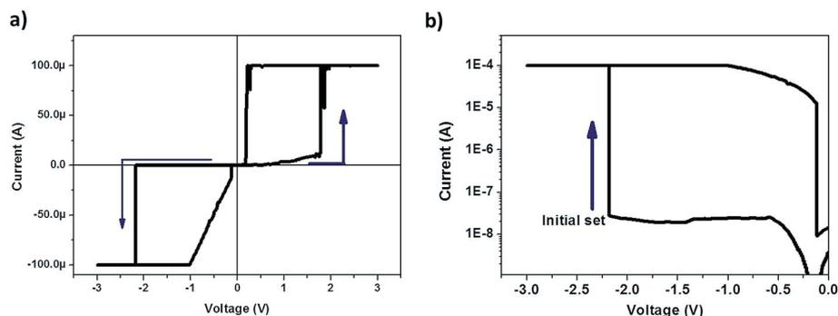
Fig. 4 (a) Initial cyclic  $I$ - $V$  measured in the Au/PAG-IL/Au system. (b) Zoom on the initial set process taking place at  $-2.2$  V.
