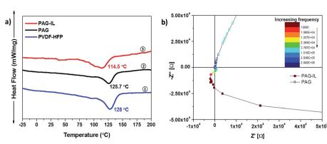
Fig. 5 (a) DSC thermograms of 1 PVDF-HFP 2 PAG and 3 PAG-IL. (b) Nyquist response of the PAG and PAG-IL analyzed from 1 kHz to 10 MHz.
