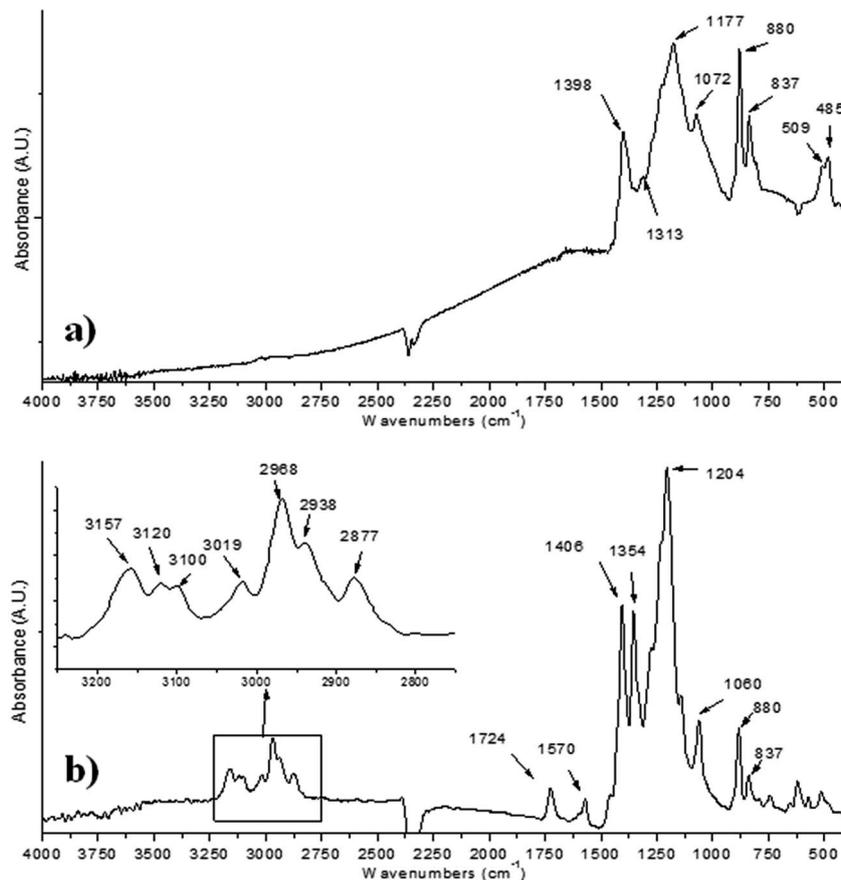
Fig. 2 ATR FTIR spectra (a) PAG (b) PAG-IL.
