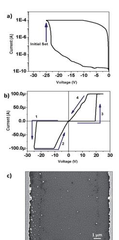
Fig. 3 (a) Initial set process, taking place at -25 V. (b) Cyclic I-V measured in the Au/PAG/Au system (c) FESEM image of the device with active switching matrix (AgNO $_3$  and PVDF-HFP) spin coated between the gold electrodes, after electrical characterization.
