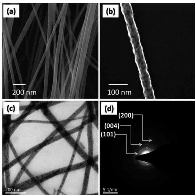
Fig. 7 FESEM image of electrospun TiO<sub>2</sub> nanofiber mat produced at 500 °C (a); (b) shows the higher magnified view of a single fiber; TEM micrograph of TiO<sub>2</sub>-nanofibers (c); and the SAED pattern presentation the crystal planes of anatase TiO<sub>2</sub> (d). Reprinted with permission from ref. 56. Copyright (2014) American Chemical Society.<sup>56</sup>
