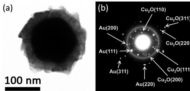
Fig. 12 (A) TEM micrograph of an individual Au–Cu<sub>2</sub>O core–shell nanoparticle with a compact metal oxide shell and (B) SAED pattern showing individual crystal planes. Reprinted with permission from ref. 155. Copyright (2012) American Chemical Society.<sup>155</sup>
