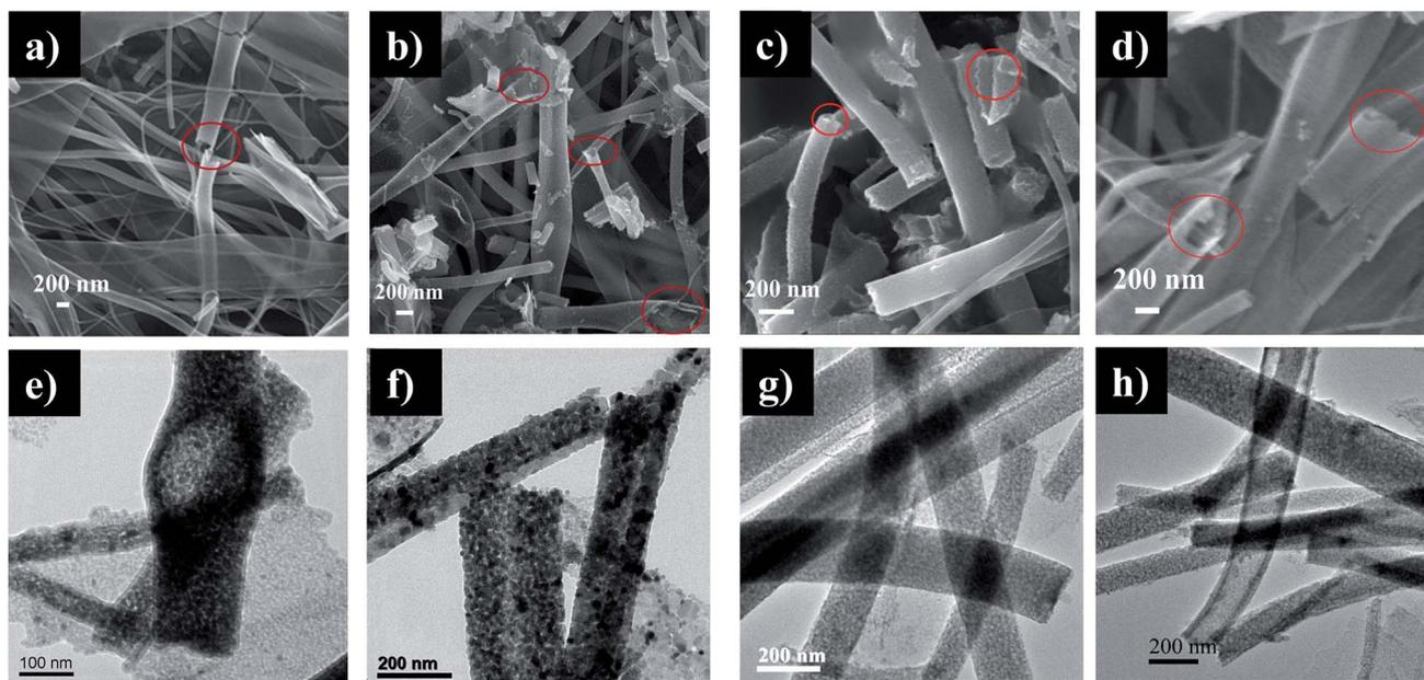
Fig. 19 FESEM images (a, b, c and d) showing CdS loaded TiO<sub>2</sub> hollow nanofibers after 1, 2, 3 and 5 SILAR cycles, respectively (marked regions show the hollow morphology of nanofibers); TEM images (e, f, g and h) reveal CdS loaded TiO<sub>2</sub> hollow nanofibers after same SILAR cycles, respectively. Reproduced with permission from ref. 198. Copyright 2016, Royal Society of Chemistry.<sup>198</sup>
