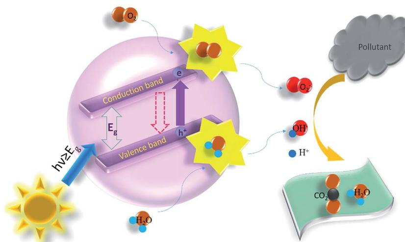
Fig. 3 The idea of degradation of pollutant by heterogeneous photocatalysis. Here, the redox potentials ( $E^0$ ) of some active radicals, such as  $H^+$ / $H_2$ ,  $O_2/O_2^-$  and  $H_2O/OH^-$  should be noted as 0 V,  $-0.33$  V and  $-0.42$  V, respectively.<sup>57</sup>
