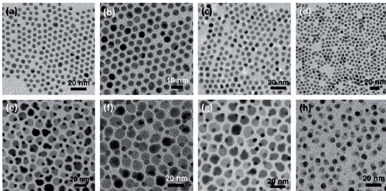
Fig. 10 TEM micrographs showing different noble metal nanoparticles: 5 nm Au (a), 5 nm Ag (b), 5 nm Pt (c), 6 nm AuAg (d); noble metal–metal oxide heterostructures of 5–12 nm Au–Fe<sub>3</sub>O<sub>4</sub> (e), 5–12 nm Ag–Fe<sub>3</sub>O<sub>4</sub> (f), 5–12 nm Pt–Fe<sub>3</sub>O<sub>4</sub> (g), and 6–10 nm AuAg–Fe<sub>3</sub>O<sub>4</sub> (h) nanoparticles. Reprinted with permission from ref. 126. Copyright (2010) American Chemical Society.<sup>126</sup>
