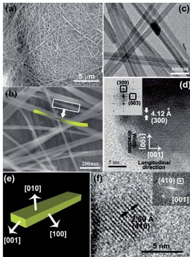
Fig. 8 Zn<sub>2</sub>GeO<sub>4</sub> nanoribbon nanostructures are described by (a and b) FESEM, (c) TEM, and (d) HRTEM images. Structural model of a nanoribbon shown in (e). (f) HRTEM micrograph imaged along [001] plane. The inset of (d) displays the FFT pattern achieved from the HRTEM micrograph. Reprinted with permission from ref. 97. Copyright (2010) American Chemical Society.<sup>97</sup>
