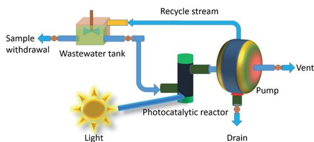
Fig. 21 Schematic diagram of a tubular photocatalytic reactor.
