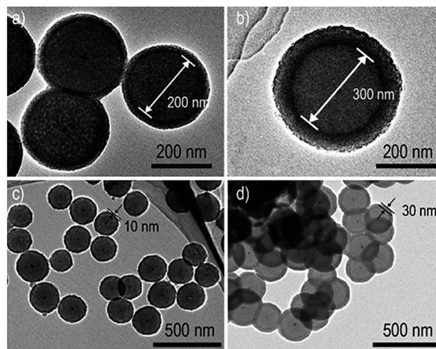
Fig. 17 TEM micrograph shows Au/carbon/Al<sub>2</sub>O<sub>3</sub> (a and b) different carbon sphere diameter and several alumina shell thickness (c and d). Reprinted with permission from ref. 163. Copyright (2015) American Chemical Society.<sup>163</sup>
