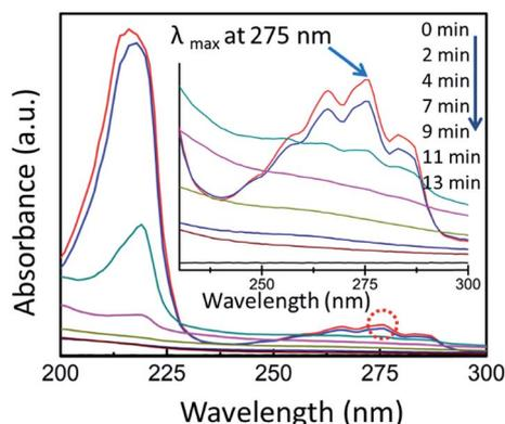
Fig. 4 Monitoring of a typical photocatalysis by UV-vis absorption spectrophotometer. Here, a typical aqueous naphthalene solution was mixed with  $TiO_2$ -NF and data collected at different time interval. The inset image shows magnified  $\lambda_{max}$  (monitored at 275 nm wavelength). Reprinted with permission from ref. 56. Copyright (2014) American Chemical Society.<sup>56</sup>
