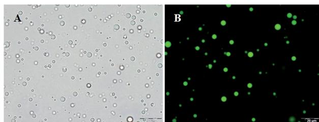
Fig. 4 Optical (A) and fluorescence (B) microscopic images of tetradecane (labelled with Nile red) filled PPI microspheres (MT-1 min). Scale: the images reported have a size of  $110 \mu\text{m} \times 147 \mu\text{m}$ .
