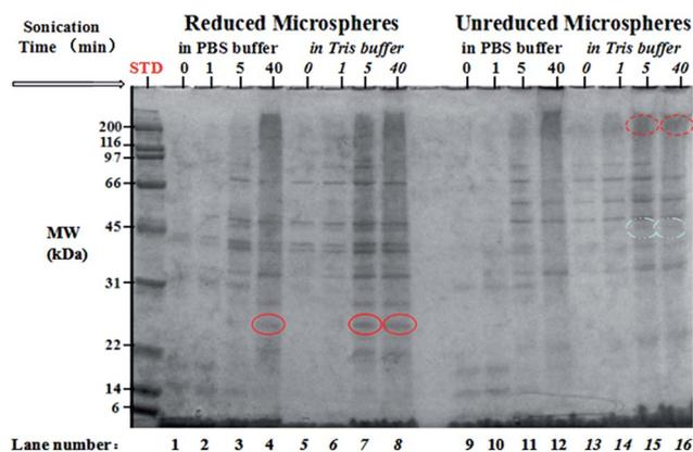
Fig. 9 SDS-PAGE profile of the PPI microspheres in PBS buffer and Tris buffer systems with sonication time. The standards (STD) were deposited in the first lane. Lanes applied by proteins in PBS buffer systems are labelled in normal font and lanes in Tris buffer systems in italic font.
