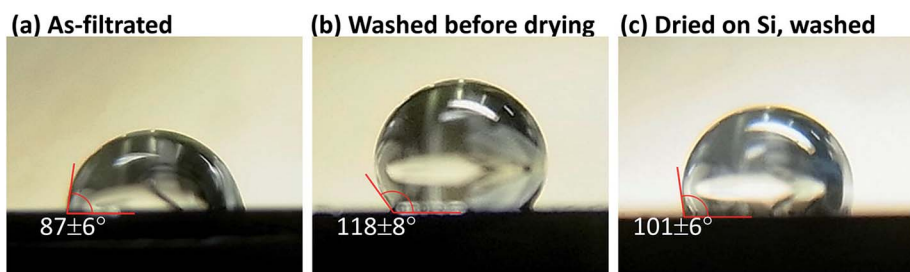
Fig. 4 Contact angle measurement of water droplets on differently-treated CNT films on flat Si substrates. The errors in the contact angles are the standard deviation for 10–12 droplets (see Fig. S4† for details).
