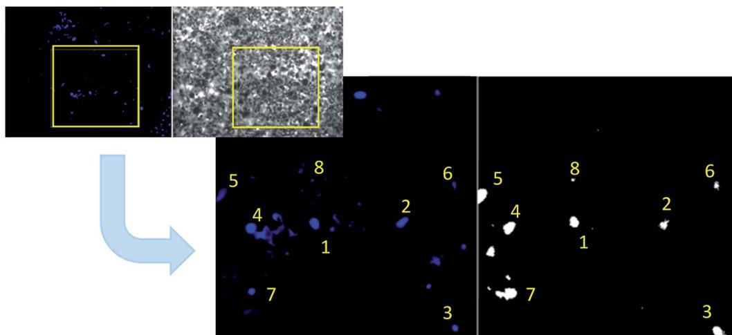
Fig. 7 Comparison of fluorescence image (wet solid fraction is stained in blue) and binary image (predicted solid fraction is presented in white area).
