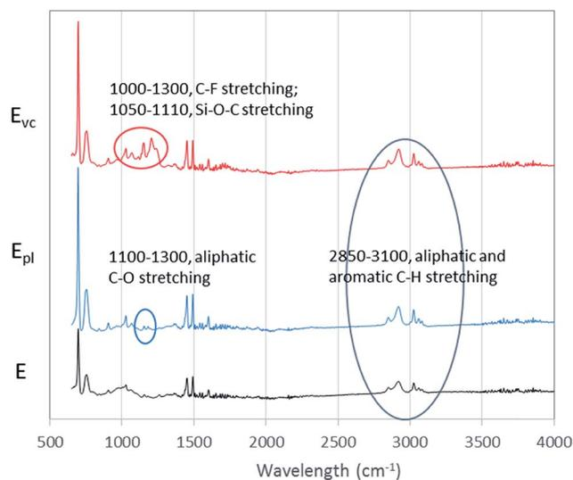
Fig. 3 FTIR spectra of PS substrates: (bottom) untreated PS electrospun web, E; (middle) PS web treated by air plasma, E<sub>pl</sub>; (top) PS web treated by air plasma followed by PFDTS vapor coating, E<sub>vc</sub>.
