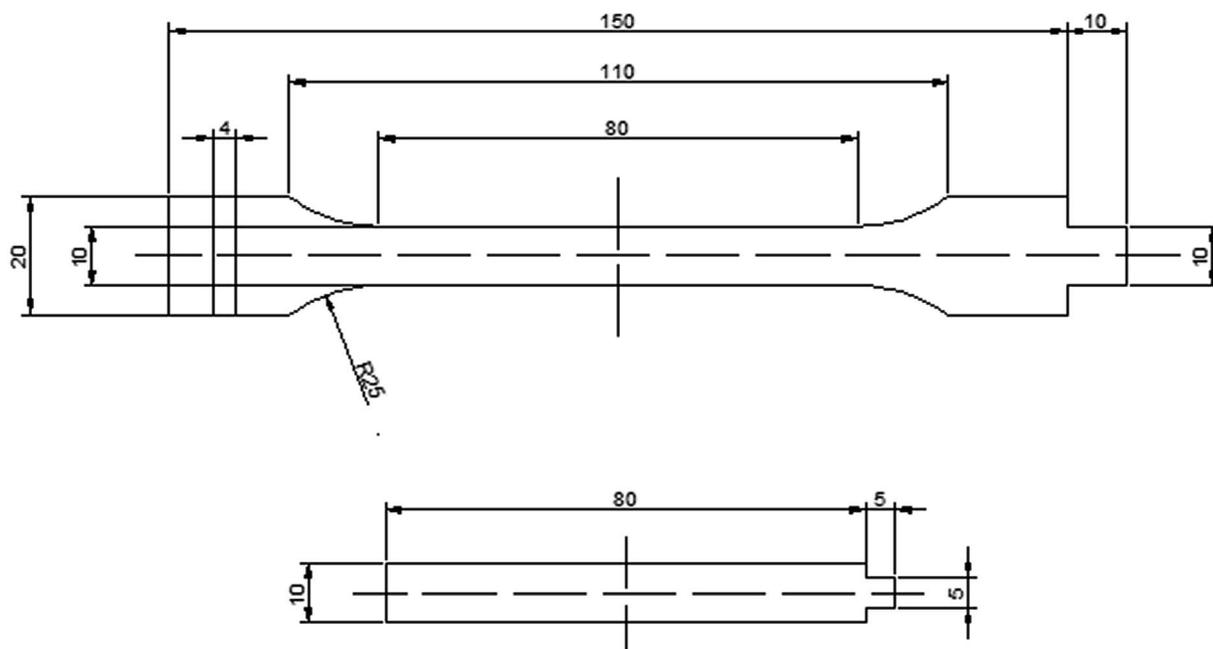
Scheme 1 The dimensions of the tensile specimens.
