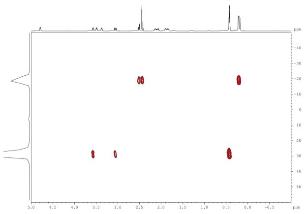
Fig. 1 Two-dimensional NMR spectrum of 9b (Bruker {<sup>1</sup>H-<sup>29</sup>Si}HMBS, CDCl<sub>3</sub>, 600 MHz).
