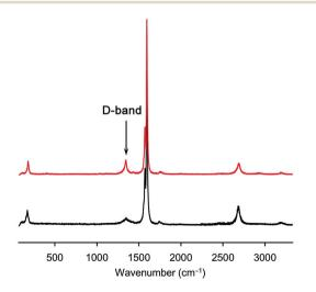
Fig. 2 Raman spectra with excitation at 532 nm of purified SWNT (black) and f-SWNT (red). The increase of the D-band at 1345 cm<sup>-1</sup> for f-SWNT is derived from the covalent functionalization with the phenylacetylene diazonium derivative.
