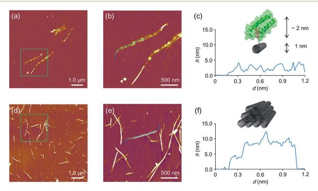
Fig. 5 AFM images of (a-c) CYT·1@f-SWNT and (d-f) f-SWNT or f-SWNT with holoCYT. Zoomed views (b and e) and height profiles (c and f) are also shown.
