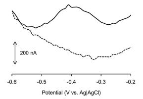
Fig. 4 DPVs of (a) CYT-1@f-SWNT and (b) f-SWNT. Scan rate: 1 to 10 V s<sup>-1</sup> in a degassed 100 mM KPi buffer (pH 7.0) at 25 °C. WE: sample + Nafion®/GC, CE: Pt mesh, RE: Ag|AgCl (3 M NaCl), 50 mM MOPS (pH 7.0), scan rate: 10 mV s<sup>-1</sup>.
