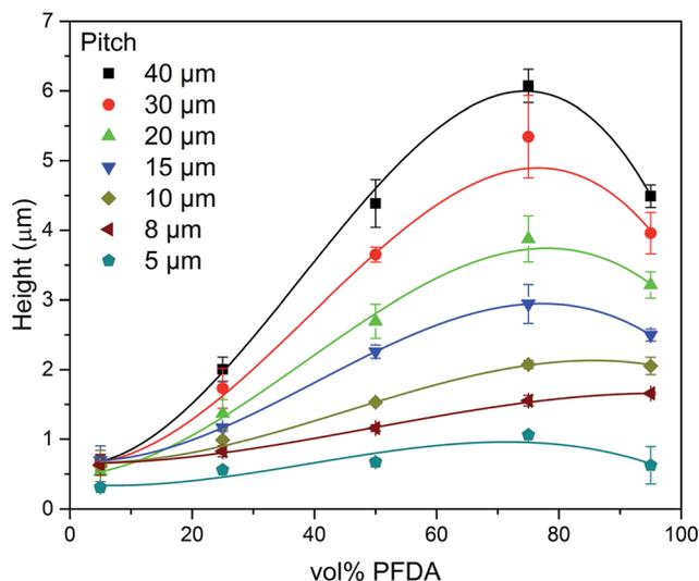
Fig. 4 Increasing the volume percentage (up to 75 vol%) of PFDA decreases the viscosity resulting in generally higher surface relief structures. However, at >95 vol% PFDA the height decreases due to the change in optical properties of the film during polymerization.
