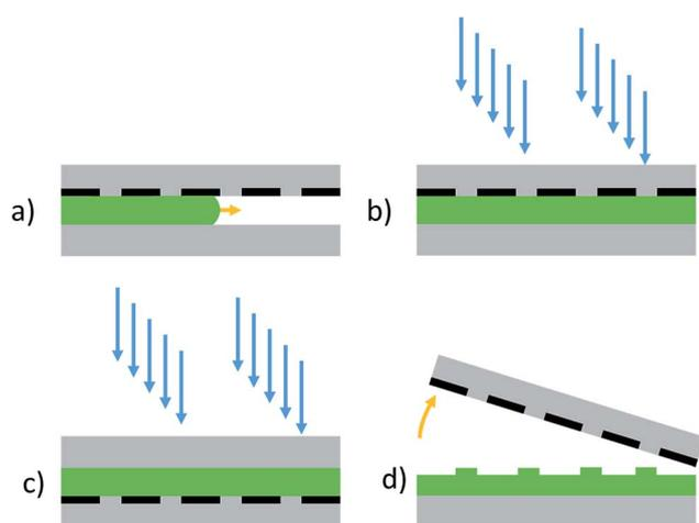
Fig. 2 Schematic representation of the method for photo-embossing liquid monomers. (a) The cell is capillary filled with the liquid monomer mixture. (b) The cell is exposed *via* the photomask and (c) subsequently a flood exposure is done *via* the substrate to polymerize the remaining monomers. (d) The photomask can then be removed by opening the cell, leaving a fluoropolymer with the desired surface relief on the substrate.
