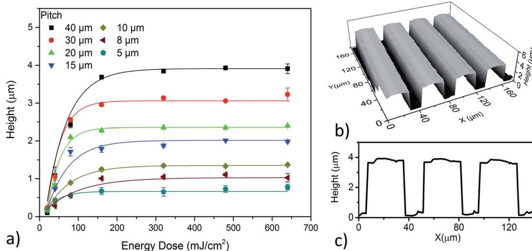
Fig. 3 (a) The height of the surface relief structures increases with increasing energy dose, until a plateau is reached after 200–250  $\text{mJ cm}^{-2}$ . The effect of the pitch of the photomask grating can also be seen, where increasing the pitch results in higher surface relief structures. An example of a typical 3D (b) and a 2D height profile (c) of structures generated using a photomask with a 40  $\mu\text{m}$  pitch and an energy dose of 640  $\text{mJ cm}^{-2}$  is shown.
