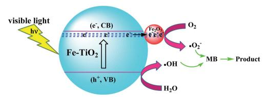
Fig. 9 The charge transfer in a Fe<sub>2</sub>O<sub>3</sub> coupled and doped TiO<sub>2</sub> photocatalyst induced degradation of MB under visible light irradiation in water.
