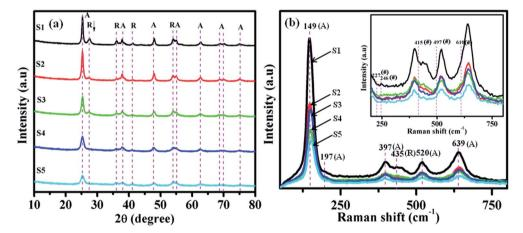
Fig. 1 XRD patterns (a) and Raman spectra (b) (insert figure short range Raman spectra) of S1–S5 samples (where A = anatase, R = rutile and # = hematite (Fe<sub>2</sub>O<sub>3</sub>)).
