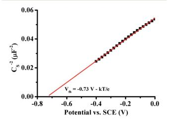
Fig. 7 Mott-Schottky plot of S5 sample obtained at frequency of 1 kHz with 0.5 M Na<sub>2</sub>SO<sub>4</sub> solution (pH 6.4), electrode area =  $0.5 \text{ cm}^2$ .
