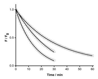
Fig. 5 Kinetic profiles of the free and protein-included Trp consumption mediated by AAPH-derived free radicals. Solutions of Trp (O), HSA ( $\square$ ), and hSOD ( $\triangle$ ) were incubated in the presence of AAPH (6 mM) in phosphate buffer at 45 °C. Trp consumption was followed by fluorescence emission at 360 nm ( $\lambda_{ex}=295$  nm). Protein concentration  $=5~\mu\text{M}$ .
