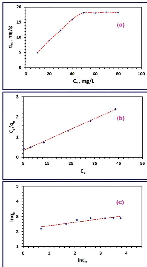
**Fig. 12** Effect of initial RR195 dye concentration (a), Langmuir isotherm model (b), and Freundlich isotherm model (c) for RR195 dye adsorption on CoFe<sub>2</sub>O<sub>4</sub> adsorbent.
