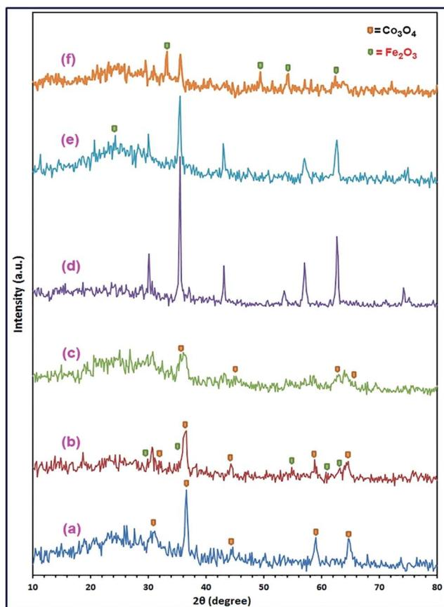
Fig. 7 XRD patterns of the calcination products; S19\_600 (a), S37\_600 (b), S46\_600 (c), S11\_600 (d), S37\_600 (e), and S91\_600 (f), of the respective  $\text{CoCO}_3/\text{FeCO}_3$  composites at 600 °C for 2 h.
