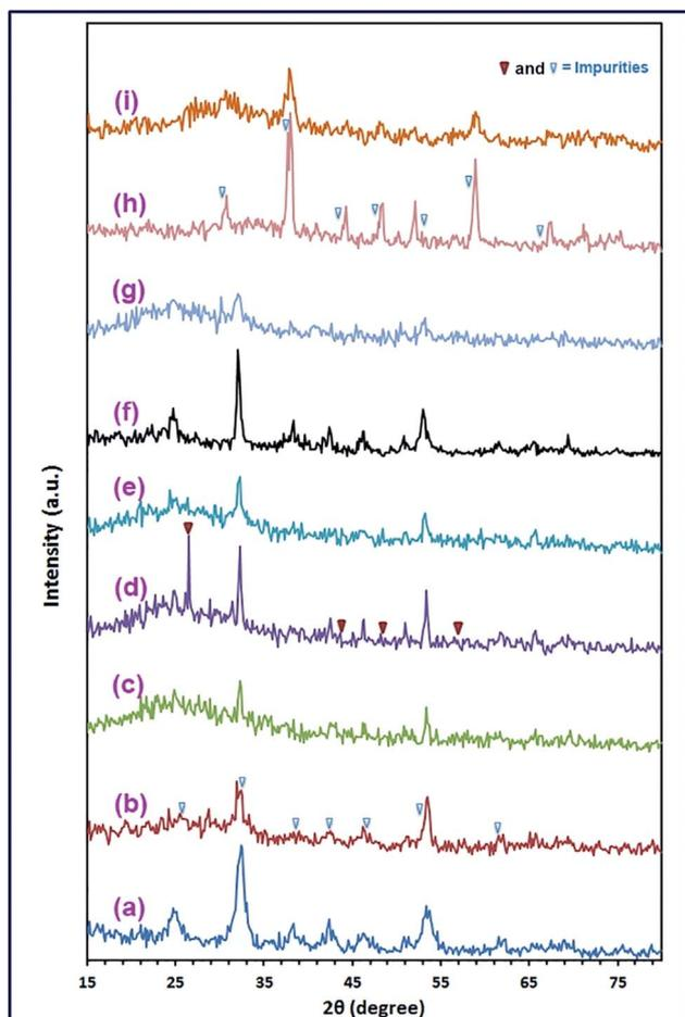
Fig. 2 XRD patterns of the as-synthesized samples; S19 (a), S28 (b), S37 (c), S46 (d), S11 (e), S64 (f), S73 (g), S82 (h), and S91 (i), with  $\text{Co}^{2+} : \text{Fe}^{2+}$  molar ratios of 0.1 : 0.9, 0.2 : 0.8, 0.3 : 0.7, 0.4 : 0.6, 0.5 : 0.5, 0.6 : 0.4, 0.7 : 0.3, 0.8 : 0.2, and 0.9 : 0.1, respectively; under hydrothermal conditions: 140 °C for 3 h.
