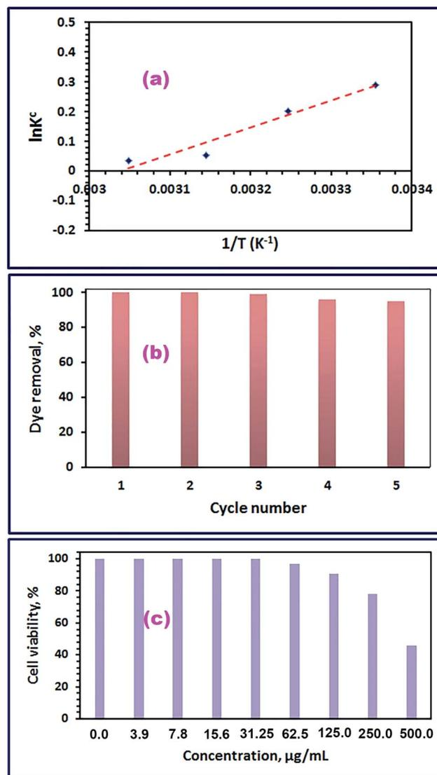
Fig. 13 Plot of  $\ln K_c$  versus  $1/T$  (a), effect of regeneration cycle on the efficiency of  $\text{CoFe}_2\text{O}_4$  adsorbent for RR195 dye removal (b), and cell viability assessment of  $\text{CoFe}_2\text{O}_4$  adsorbent at pH 2 (c).
