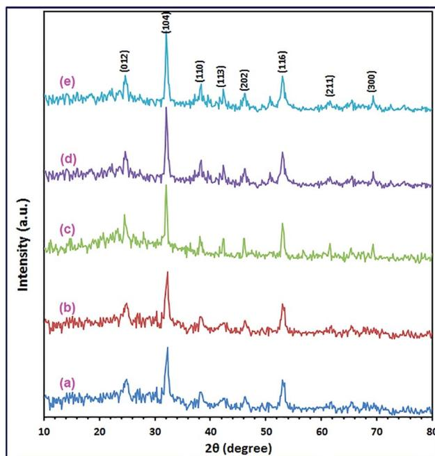
Fig. 3 XRD patterns of the as-synthesized  $\text{CoCO}_3/\text{FeCO}_3$  composites under hydrothermal reactions:  $\text{Co}^{2+} : \text{Fe}^{2+} : \text{ascorbic acid} : \text{CO}_3^{2-}$  molar ratio of 0.4 : 0.6 : 1 : 3, respectively, at 140 °C, for varying reaction times of 1.5 (a), 3 (b), 6 (c), 12 (d), and 24 h (e).
