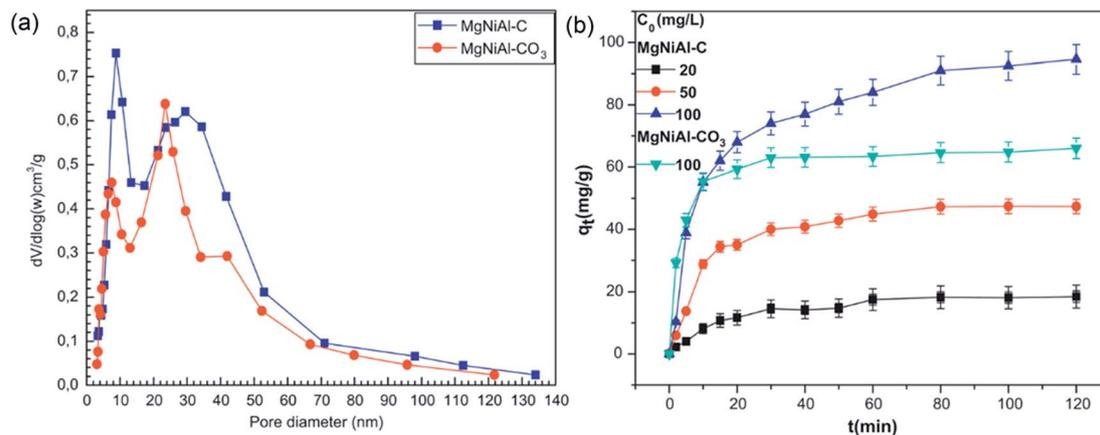
Fig. 9 The pore size distribution curves (a) and effect of time and initial concentration and (b) in the adsorption of MO on the two samples (adapted from ref. 58 with Copyright from 2012 Elsevier).
