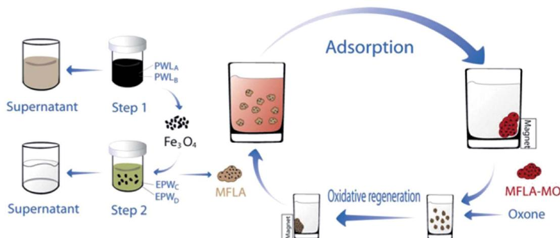
Fig. 8 Synthesis route of MFLA and their application for removal of MO with the help of an external magnetic field (MFLA: magnetic Fe<sub>3</sub>O<sub>4</sub>/Zn–Cr LDH adsorbent, PWL: pickling waste liquor, EPW: electroplating wastewater). Adapted from ref. 70 with Copyright from 2012 Elsevier.
