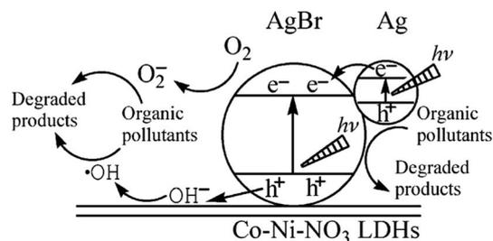
Fig. 14 Schematic photocatalytic mechanism of Ag/AgBr/Co-Ni-NO<sub>3</sub> LDH nanocomposites under visible-light illumination (adapted from ref. 149 with Copyright from 2013 Wiley).
