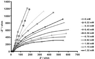
Fig. 3 Nyquist plots of  $Ni(OH)_2$  thin film on Au electrode in 0.1 M KOH solution for glucose in the 0–1.32 mM concentration scope. Adapted with permission from ref. 69. Copyright @ 2016 Elsevier B.V.
