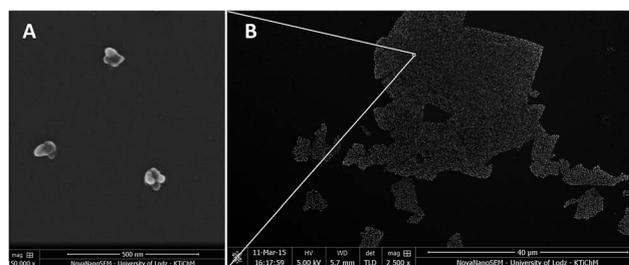
Fig. 4 SEM image (magnification 150 000 $\times$ ) presenting the morphology of AgNPs on RGO flakes (A) taken from a low-magnification image (2500 $\times$ ) presenting the general view of RGO flakes with AgNPs deposited on silicon wafer (B). AgNPs were grown only at RGO.
