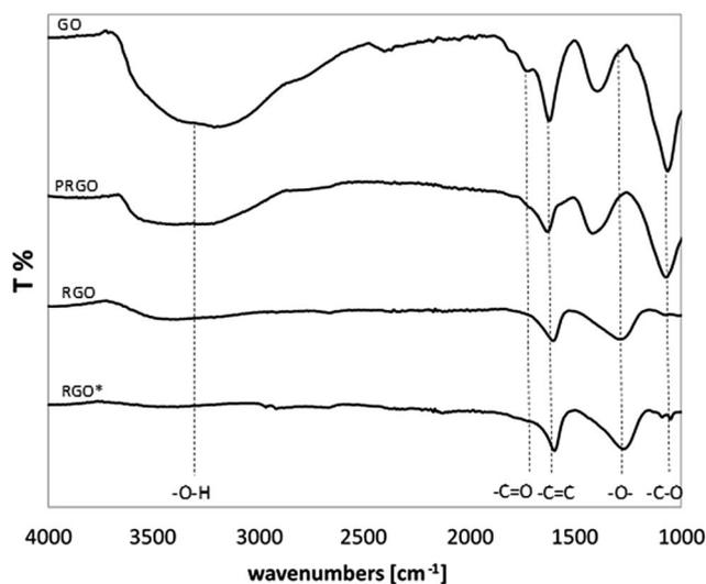
Fig. 2 FT-IR spectra of GO, PRGO and RGO.
