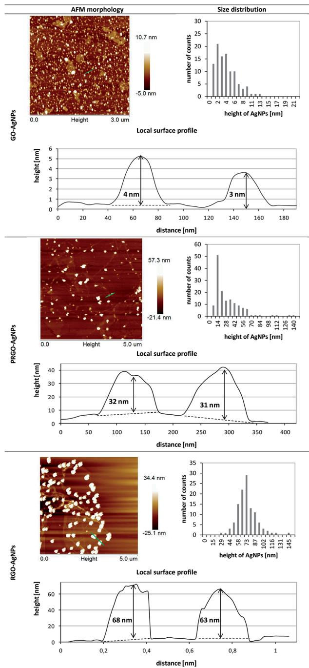
Fig. 6 Surface morphology and distribution of AgNPs on GO, PRGO and RGO imaged by AFM.
