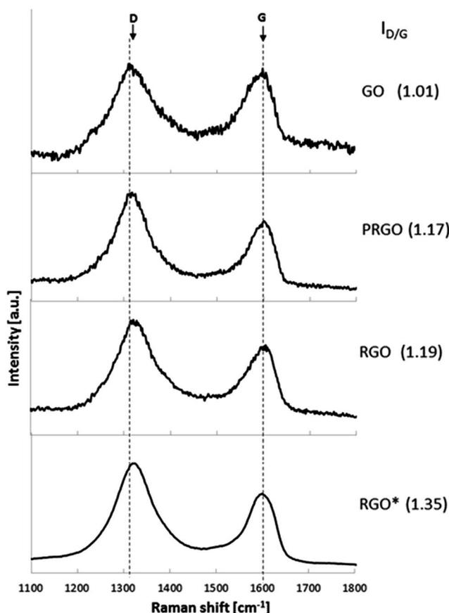
Fig. 3 Raman spectra of GO, PRGO and RGO.
