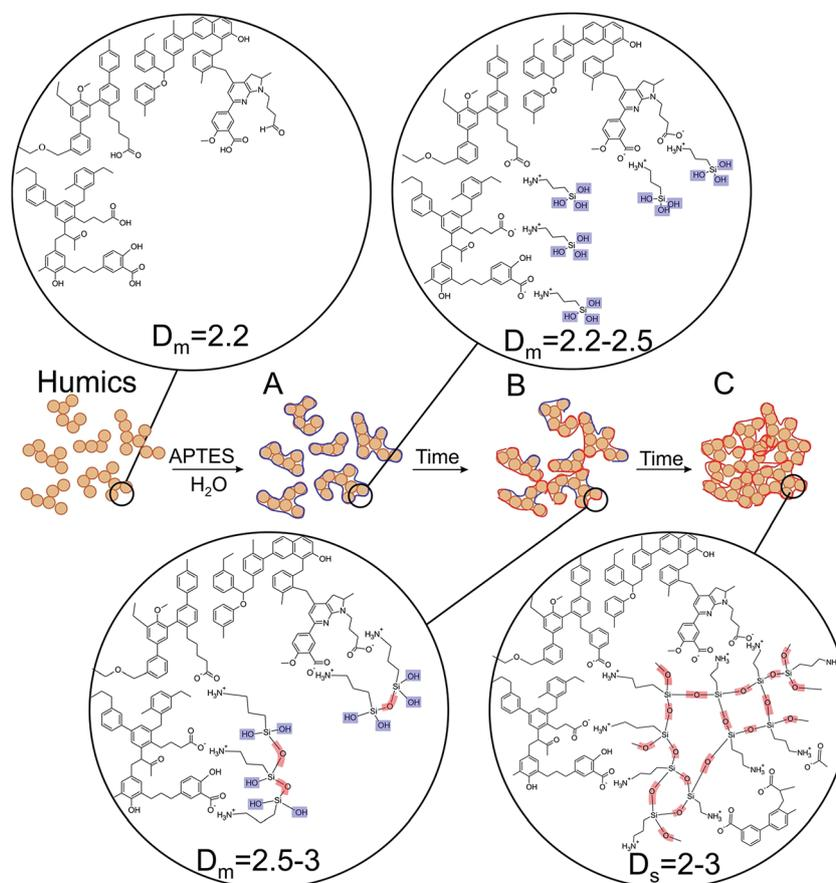
Fig. 3 Conceptual model of the water-based HS-SQ network formation and evolution in time: the first insert shows a fragment of HS network with  $D_m$  of 2.2, (A) shows formation of CHP-APTES complexes rich in silanol groups (marked in blue) with low  $D_m$  values, (B) shows initial siloxane bonding (marked in red) resulting in aggregate formation with high  $D_m$  values, (C) shows branched silsesquioxane cross-linking ( $D_m$  to  $D_s$  transition).
