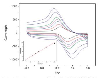
Fig. 3 Cyclic voltammograms of the Apt/Fc@WMCNTs/OMC/GCE in 0.1 M PBS (pH 7.0) at scan rates (from inner to outer) 20, 40, 60, 80, 100, 150 and 200 mV s $^{-1}$ , respectively. Inset: the relationship between scan rates and peak currents.
