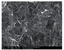
Fig. 1 SEM images of (A) OMC, (B) Fc-MWNTs, (D) Fc-MWNTs/OMC; (C) EDS for Fe elemental distribution on the surface of Fc@MWNTs.
