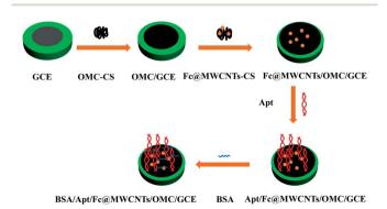
Scheme 1 Stepwise preparation of the aptasensor.
