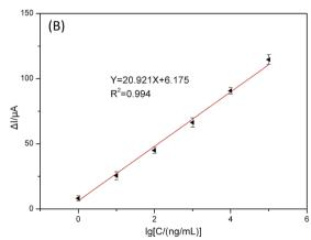
Fig. 5 The CVs (A) of the aptasensor after incubation in different concentrations of chlorpyrifos standard solution (from a to f):  $10^5$ ,  $10^4$ , 1000, 100, 10, 1 ng mL $^{-1}$  under the optimal conditions; and the calibration curve (B) of the relative current changes ( $\Delta I$ ) of the proposed aptasensor *versus* the logarithm of chlorpyrifos concentrations.
