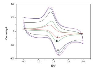
Fig. 2 CVs of modified GCE recorded in 0.1 M PBS (pH 7.0) containing 5.0 mM  $[Fe(CN)_6]^{3-/4-}$  and 0.1 M KCI: (a) bare GCE; (b) OMC/GCE; (c) Fc@MWCNTs/OMC/GCE; (d) Apt/Fc@MWCNTs/OMC/GCE; (e) BSA/Apt/Fc@MWCNTs/OMC/GCE.
