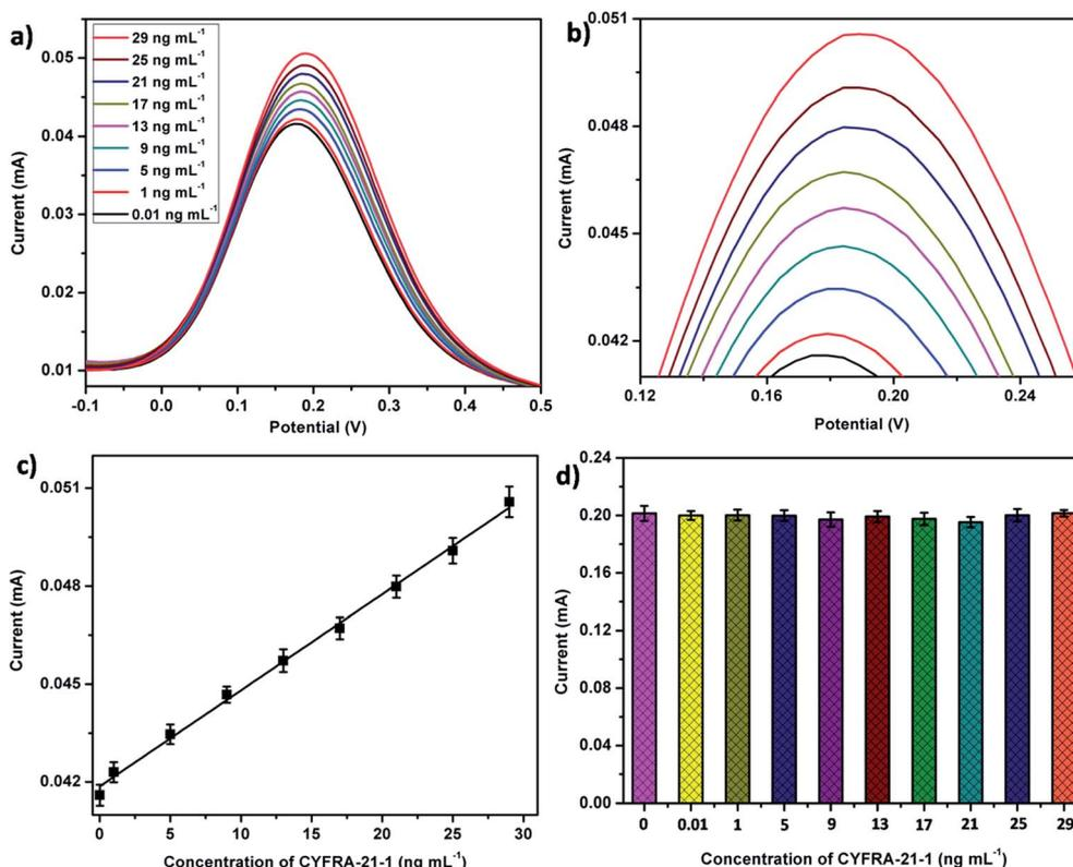
Fig. 5 (a) DPV response studies of BSA/anti-CYFRA-21-1/serine/nZrO<sub>2</sub>/ITO immunoelectrode as a function of CYFRA-21-1 concentration (0.01–29 ng mL<sup>-1</sup>), (b) magnified view of peak current response, (c) calibration curve between the magnitude of peak current and concentration of CYFRA-21-1 (ng mL<sup>-1</sup>) and (d) A control experiment of serine/nZrO<sub>2</sub>/ITO electrode as a function of CYFRA-21-1 concentration (0.01–29 ng mL<sup>-1</sup>).
