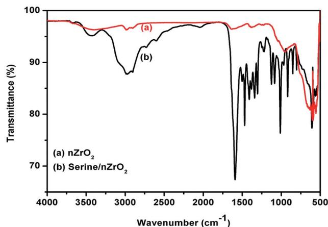
Fig. 2 FTIR spectra of (a) nZrO<sub>2</sub> nanoparticles and (b) serine functionalized nZrO<sub>2</sub> nanoparticles (serine/nZrO<sub>2</sub>).
