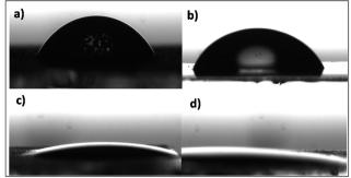
Fig. 4 Contact angle measurements of (a) ITO (b) APTES/nZrO<sub>2</sub>/ITO (c) serine/nZrO<sub>2</sub>/ITO and (d) anti-CYFRA-21-1/serine/nZrO<sub>2</sub>/ITO electrodes.
