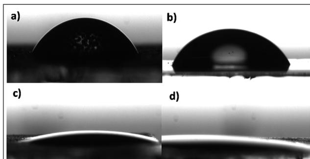
Fig. 4 Contact angle measurements of (a) ITO (b) APTES/nZrO<sub>2</sub>/ITO (c) serine/nZrO<sub>2</sub>/ITO and (d) anti-CYFRA-21-1/serine/nZrO<sub>2</sub>/ITO electrodes.
