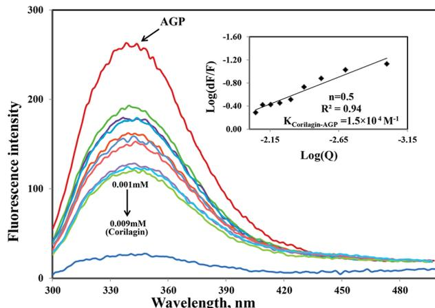
Fig. 2 Fluorescence emission spectra were measured for AGP along with corilagin in 0.1 M phosphate buffer with pH 7.2,  $\lambda_{\text{ex}} = 285$  nm, and temperature =  $25 \pm 1$  °C. Free AGP (0.001 mM) and free AGP with different concentrations of corilagin, 0.001–0.009 mM. Insert: plot of  $\log(dF/F)$  against  $\log[Q]$ .  $\lambda_{\text{ex}} = 285$  nm and  $\lambda_{\text{em}} = 340$  nm.
