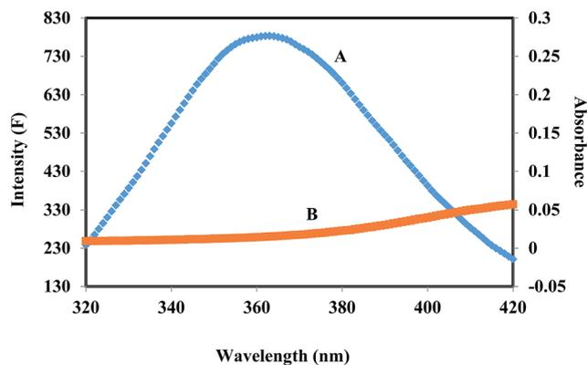
Fig. 3 The overlap of fluorescence spectrum of HSA (A) and absorbance spectrum of corilagin (B) [ $\lambda_{\text{ex}} = 285 \text{ nm}$ ,  $\lambda_{\text{em}} = 360 \text{ nm}$   $c(\text{HSA})/c(\text{corilagin}) = 1 : 1$ ].
