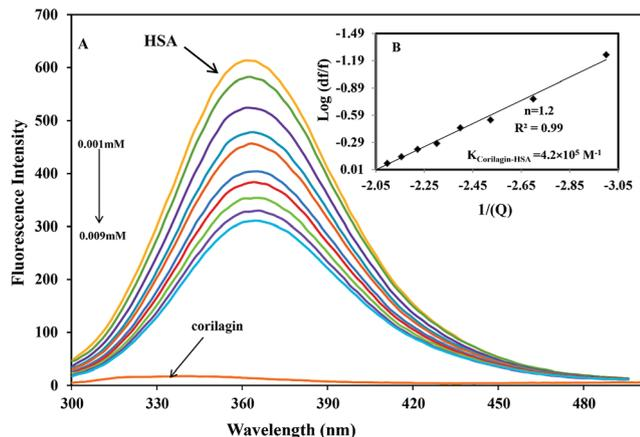
Fig. 1 Fluorescence emission spectra of HSA–corilagin in 0.1 M phosphate buffer with pH 7.2,  $\lambda_{\text{ex}} = 285$  nm, and temperature =  $25 \pm 1$  °C. (A) Free HSA (0.001 mM) and free HSA with different concentrations corilagin of 0.001–0.009 mM. (B) Plot of  $\log(dF/F)$  against  $\log[Q]$ .  $\lambda_{\text{ex}} = 285$  nm and  $\lambda_{\text{em}} = 360$  nm.
