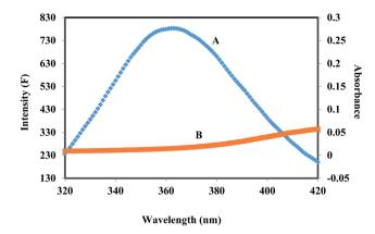
Fig. 3 The overlap of fluorescence spectrum of HSA (A) and absorbance spectrum of corilagin (B) [ $\lambda_{ex} = 285$  nm,  $\lambda_{em} = 360$  nm c(HSA)/c(corilagin) = 1:1].
