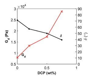
Fig. 11 Dynamic shear modulus and phase shift for P(3HB) : PBAT 20 : 80 blends with addition of DCP measured by rheology at 1 Hz and 180  $^{\circ}$ C.
