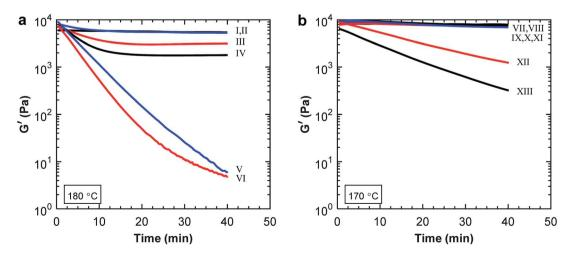
Fig. 6 Shear storage modulus measured by rheology at the processing temperatures of (a) P(3HB): PBAT blends [0:100 (I), 20:80 (II), 40:60 (III), 60:40 (IV), 80:20 (V) and <math>100:0 (VI), and 100:0 (VI), and 100:0 (VI), and 100:0 (VIV).
