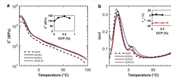
Fig. 12 Tensile storage modulus (a) and  $\tan \delta$  (b) for P(3HB): PBAT 20: 80 blends with addition of DCP. The inset in part (a) shows the change in E' with the content of DCP, and the inset in part (b) shows the  $T_q$  of P(3HB) ( $\bullet$ ) and PBAT ( $\mathbf{x}$ ) determined from the loss modulus peak value.
