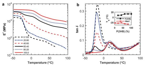
Fig. 7 Tensile storage modulus (a) and  $\tan \delta$  (b) of the P(3HB) : PBAT blends. The inset presents the  $T_g$  of P(3HB) and PBAT in the blends determined from the position of the loss modulus peak.
