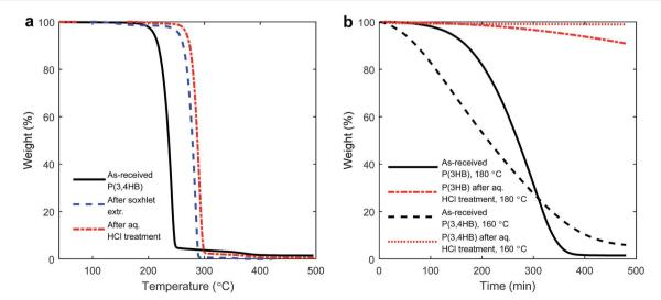
Fig. 1 TGA traces of as-received and pre-treated P(3,4HB) recorded at 10 °C min<sup>-1</sup> under nitrogen (a) and TGA traces showing the isothermal decomposition of P(3,4HB) and P(3HB) materials under air during 8 h at 160 and 180 °C, respectively (b).
