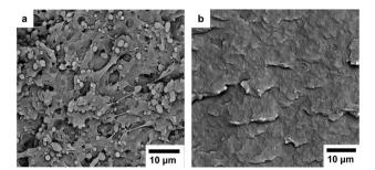
Fig. 8 SEM images of cryo-fractured surfaces of P(3HB): PBAT 20: 80 blends (a) without DCP and (b) with 0.5 wt% DCP added.
