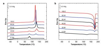
Fig. 5 DSC traces of the P(3HB): PBAT blends: cooling (a) and second heating scans (b).
