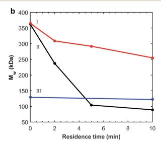
Fig. 2 Degradation observed by (a) monitoring the melt shear storage modulus of P(3,4HB): (I) treated with aq. HCl solution, (II) soxhlet extracted with CHCl<sub>3</sub> and (III) as-received, and by (b) following the molecular weight measured by SEC of (I) HCl-treated P(3,4HB), (II) as-received P(3,4HB) and (III) PBAT.
