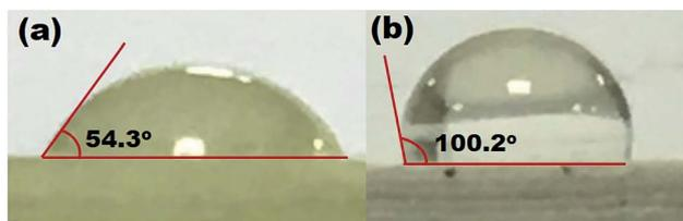
Fig. 5 Contact angle of water on the surface of a (a) AP (b) APD-30 composite.
