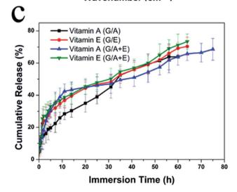
Fig. 3 (a) XRD patterns of vitamin E TPGS and the cross-linked nanofibers prepared in this work; (b) FTIR spectra of the cross-linked fibers; (c) the *in vitro* vitamin release profiles from the G/A, G/E and G/A + E fibers.
