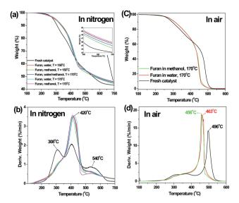
Fig. 9 TGA and DTG curves for the used catalyst (polymer plus catalyst) and fresh Amberlyst 70 catalyst. The fresh catalyst and the used catalysts were dried at 100 °C in nitrogen for 60 min before further heating to 700 °C in nitrogen and 600 °C in air at 10 °C min $^{-1}$ . The gas flow rate was 100 mL min $^{-1}$ . Typical reaction conditions experienced by the catalysts are described inside the figures. Detailed conditions are specified in the caption of Fig. 5.
