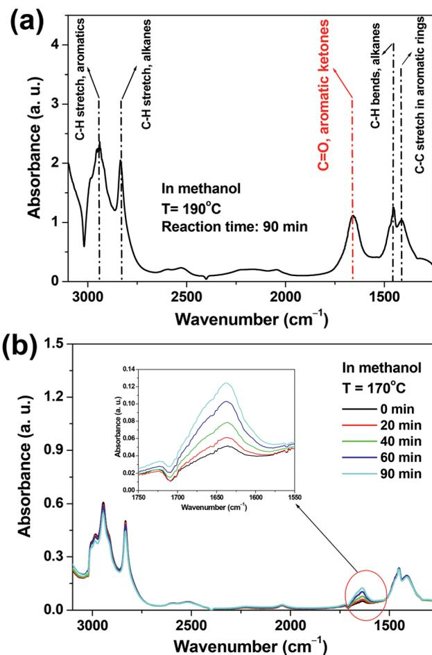
Fig. 3 The FT-IR characterization of the liquid samples from the acid-treatment of furan in methanol at (a)  $T = 190\text{ }^{\circ}\text{C}$  and (b)  $T = 170\text{ }^{\circ}\text{C}$ . The sample in Fig. 4a was analyzed directly without dilution. The samples in Fig. 4b were diluted to 10 wt% in chloroform before the analysis.
