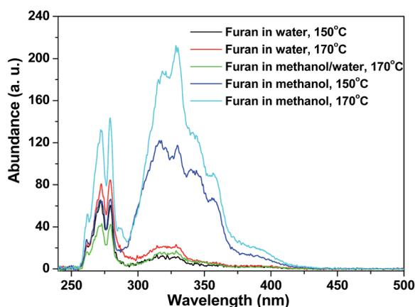
Fig. 8 Constant energy ( $-2800\text{ cm}^{-1}$ ) synchronous spectra for the soluble polymers in the liquid samples. The typical reaction conditions are described inside the figure. Detailed conditions are specified in the caption of Fig. 5.
