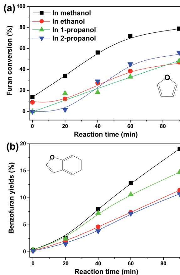
**Fig. 10** The conversion of furan in the alcohols. (a) Furan conversion in the alcohols; (b) the yields of benzofuran in the alcohols. Reaction conditions: furan, 3 g; solvent, 100 ml; catalyst, A70, 3 g; stirring rate, 350 rpm; reaction time, 90 min; pressure, autogenous vapor pressure. "0 min" in the x-axis means the reaction temperature just reached the required temperature.
