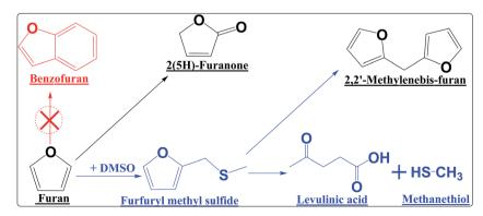
Scheme 4 A proposed reaction network for the conversion of furan in DMSO. All the compounds listed above were detected with GC-MS.
