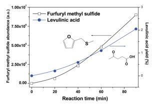
Fig. 12 The formation of levulinic acid and furfuryl methyl sulfide in acid treatment of furan in DMSO.
