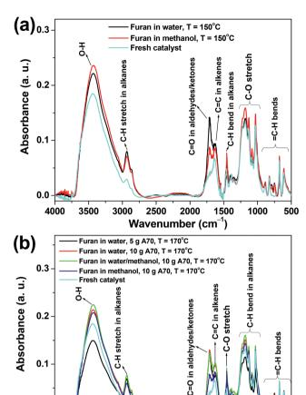
Fig. 6 FT-IR spectra of the fresh Amberlyst 7 and the used catalysts (polymer plus catalyst) obtained at (a) 150 °C and (b) 170 °C. The typical reaction conditions for the catalysts experienced were described inside figures. The detailed conditions can refer to that specified in the caption of Fig. 5.
