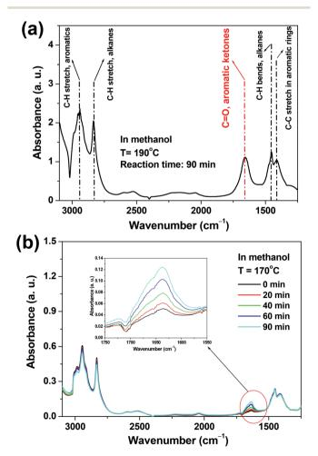
Fig. 3 The FT-IR characterization of the liquid samples from the acid-treatment of furan in methanol at (a)  $T=190\,^{\circ}\text{C}$  and (b)  $T=170\,^{\circ}\text{C}$ . The sample in Fig. 4a was analyzed directly without dilution. The samples in Fig. 4b were diluted to 10 wt% in chloroform before the analysis.
