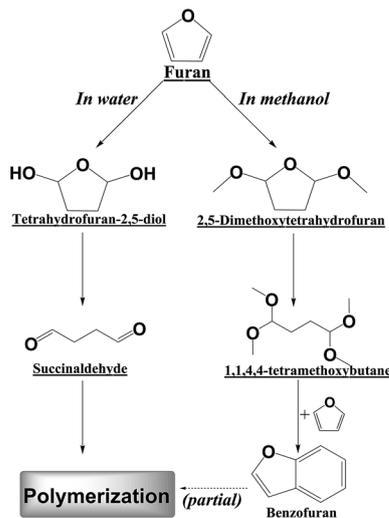
**Scheme 1** The distribution of the main products during the conversion of furan in water and in methanol. All the compounds listed above except the polymer were detected with GC-MS. Tetrahydrofuran-2,5-diol, succinaldehyde, 2,5-dimethoxytetrahydrofuran and 1,1,4,4-tetramethoxybutane are the intermediates. The opening of the furan ring, the acetalization, the formation of benzofuran and the polymer were believed to be the acid-catalyzed reactions.
