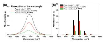
Fig. 7 (a) FT-IR spectra of the soluble polymers; (b) deconvolutions of the FT-IR spectra in Fig. 7a. The liquid products were diluted to 50% (by volume) with methanol before the characterization with FT-IR.
