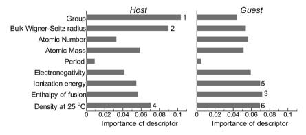
Fig. 6 Feature-importance scores of the descriptors for the GBR prediction of the d-band centers for the surface monolayer of guest metals on the host metals.
