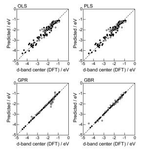
Fig. 1 DFT calculated local d-band center for metals and 1% guest metal-doped metals (Table 1) and the values predicted by linear (OLS, PLS) and nonlinear regression (GPR, GBR): ( $\bullet$ ) training set = 75%, ( $\bigcirc$ ) test set = 25%.
