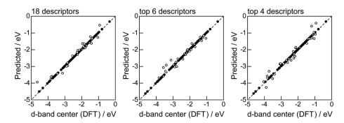
Fig. 7 DFT calculated local d-band center for the surface monolayer of guest metals on the host metals (Table 2) and the values predicted by GBR with the 18 (all), top 6, and top 4 descriptors in Fig. 6: (●) training set = 75%, (○) test set = 25%.
