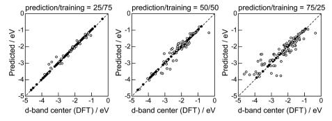
Fig. 8 DFT calculated local d-band center for the surface monolayer of guest metals on the host metals (Table 2) and the values predicted by GBR with the top 6 descriptors: (♠) training set, (○) test set.
