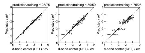
Fig. 4 DFT calculated local d-band center for 1% guest metals on the surface of host metals and the values predicted by GBR with the top 6 descriptors: (●) training set, (○) test set.
