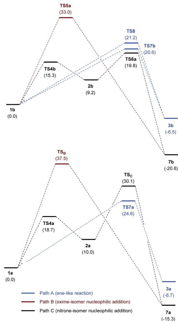
Fig. 7 Comparative free energy diagrams (M06-2X/cc-pVTZ/PCM = EtOH) for the reaction between **1b** and **6** (top) and **1a** and **6** (bottom). Relative free energies are given in kcal mol<sup>-1</sup>.
