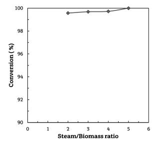
Fig. 6 Effect of S/B ratio on conversion. Reforming conditions:  $600\,^{\circ}\text{C}$ ; space time,  $20\,\,\text{g}_{\text{cat}}$  min  $\text{g}_{\text{volatiles}}^{-1}$ .
