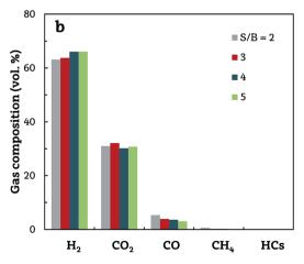
Fig. 7 Effect of S/B ratio on the yields of the gaseous products (a) and their concentrations (on a dry basis) (b). Reforming conditions:  $600\,^{\circ}\text{C}$ ; space time,  $20\,_{\text{gcat}}$  min  $g_{\text{volatiles}}^{-1}$ .
