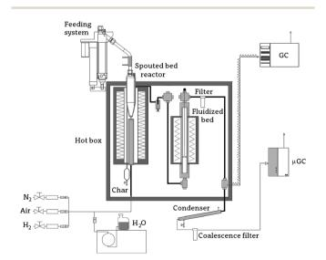
Fig. 1 Scheme of the laboratory scale pyrolysis-reforming plant.
