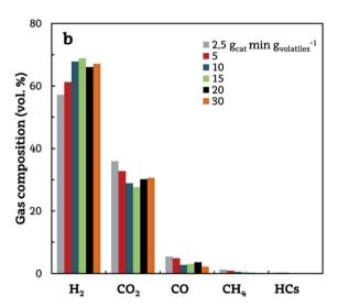
Fig. 5 Effect of reforming space time on the yields of gaseous products (a) and their concentrations (on a dry basis) (b). Reforming conditions:  $600 \,^{\circ}\text{C}$ ; S/B ratio, 4.
