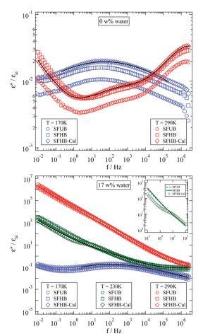
Fig. 7 Normalised dielectric loss measured at different water levels and temperatures for all three investigated types of paper. The inset shows the increased  $\beta_{wet}$ -relaxation strength of the SFHB-Cal sample. Solid lines are fits of the model described in Section 2.4 to the SFHB-Cal sample data.
