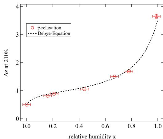
Fig. 11 Relaxation strength  $\Delta\epsilon$  of the  $\gamma$ -relaxation at 210 K against relative humidity during previous sample storage. The dashed line is a scaled estimation of the relaxation strength based on the weighing experiments (see text for details).
