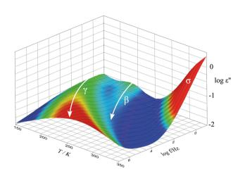
Fig. 5 Imaginary part  $\varepsilon''$  of the dielectric function of the SFHB-Cal paper sample in the completely dried state.
