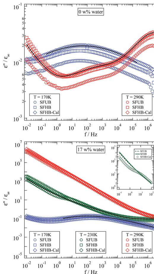
Fig. 7 Normalised dielectric loss measured at different water levels and temperatures for all three investigated types of paper. The inset shows the increased  $\beta_{\text{wet}}$ -relaxation strength of the SFHB-Cal sample. Solid lines are fits of the model described in Section 2.4 to the SFHB-Cal sample data.
