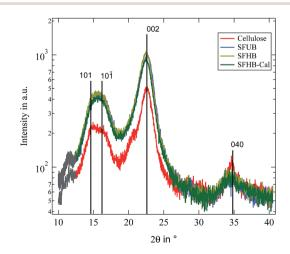
Fig. 2 Recorded WAXS patterns for all investigated paper samples as well as microcrystalline cellulose. Black lines indicate expected peak positions.<sup>22</sup> Grey part of the curves is due to background scattering from the sample holder.
