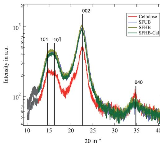
Fig. 2 Recorded WAXS patterns for all investigated paper samples as well as microcrystalline cellulose. Black lines indicate expected peak positions.<sup>22</sup> Grey part of the curves is due to background scattering from the sample holder.
