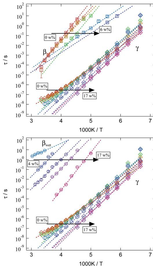
Fig. 13 Arrhenius representation of the mean relaxation times of the three analysed relaxations for different water contents in the SFHB-Cal sample. For clarification  $\beta$ - and  $\beta_{\text{wet}}$ -relaxation are given separately, while the  $\gamma$ -relaxation is the same in both tiles. Colour code is identical to Fig. 8.
