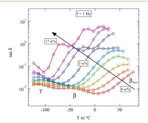
Fig. 8 Loss tangent  $\tan\delta$  measured at 1 Hz of the differently humidified SFHB-Cal sample. Arrow indicates increasing weight percent of water.
