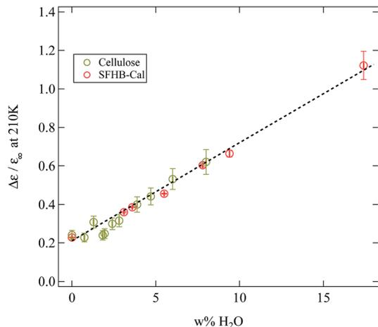
Fig. 12 Normalised relaxation strength of the  $\gamma$ -relaxation at 210 K plotted against the mass fraction of water present in the sample. A linear dependency independent from the sample type can be seen.
