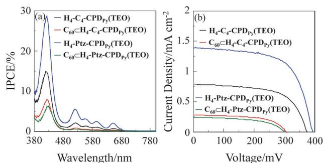
Fig. 5 (a) IPCE spectra and (b) *I*-*V* curves of DSSCs based on **H<sub>4</sub>-C<sub>4</sub>-CPD<sub>Py</sub>(TEO)**, **C<sub>60</sub>⊂H<sub>4</sub>-C<sub>4</sub>-CPD<sub>Py</sub>(TEO)**, **H<sub>4</sub>-Ptz-CPD<sub>Py</sub>(TEO)**, and **C<sub>60</sub>⊂H<sub>4</sub>-Ptz-CPD<sub>Py</sub>(TEO)**.
