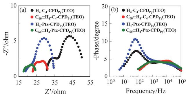
Fig. 6 (a) Nyquist plots and (b) Bode phase plots of DSSCs based on **H<sub>4</sub>-C<sub>4</sub>-CPD<sub>Py</sub>(TEO)**, **C<sub>60</sub>⊂H<sub>4</sub>-C<sub>4</sub>-CPD<sub>Py</sub>(TEO)**, **H<sub>4</sub>-Ptz-CPD<sub>Py</sub>(TEO)**, and **C<sub>60</sub>⊂H<sub>4</sub>-Ptz-CPD<sub>Py</sub>(TEO)**.
