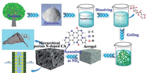
Scheme 1 Illustration of the preparations and applications of hierarchical porous N-doped carbon aerogel.
