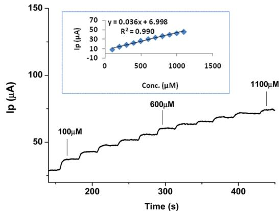
Fig. 7 Calibration curve showing  $I_p$  vs. time amperometric analysis for various concentrations of urea in the range of 100–1100  $\mu\text{M}$  (inset shows corresponding linear regression plot).
