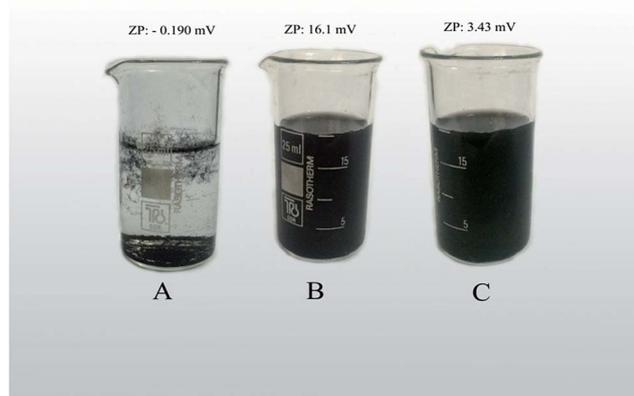
Fig. 1 Stability of different colloidal dispersions in water after 6 months: (a) pristine FGN, (b) 10  $\text{mg ml}^{-1}$  FGN/CTAB colloidal dispersion, (c) 20  $\text{mg ml}^{-1}$  FGN/CTAB colloidal dispersion.
