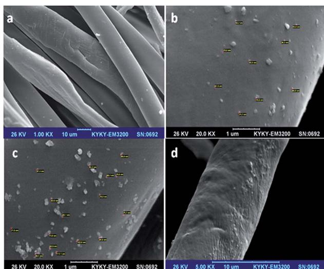
Fig. 6 SEM micrographs of: (a) untreated cotton, (b) cotton coated with 10 cycles of 10 mg ml<sup>-1</sup> FGN/CTAB colloidal dispersion and polyvinylphosphonic acid, (c) cotton coated with 10 cycles of 20 mg ml<sup>-1</sup> FGN/CTAB colloidal dispersion and polyvinylphosphonic acid, (d) cotton coated with polyvinylphosphonic acid.
