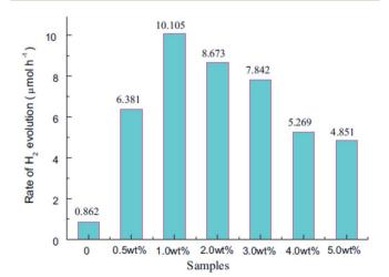
Fig. 22 Photocatalytic activity of  $Ag/g-C_3N_4$  composites for  $H_2$  evolution from methanol solution under visible light (reproduced from ref. 61).
