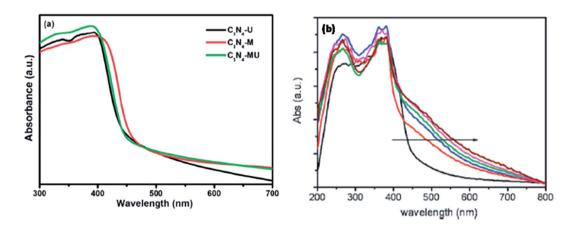
$\textbf{Fig. 15} \quad \textbf{(a) UV-Vis DRS of neat } g-C_3N_4 \text{ and (b) mesoporous } g-C_3N_4 \text{ prepared by using different amounts of P123 (reproduced from ref. 3 and 30)}.$
