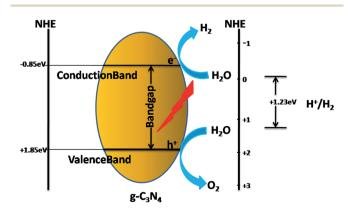
Scheme 1 Charge transfer mechanism of neat  $g\text{-}C_3N_4$  as a photocatalyst.
