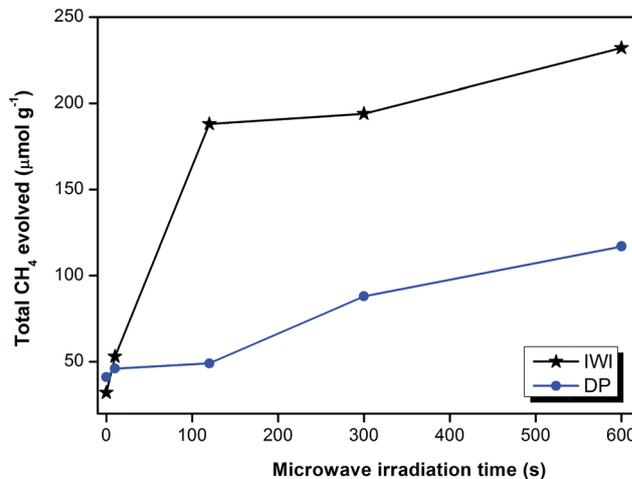
Fig. 5 Total CH<sub>4</sub> produced in the TPSR by the 1.0K/10Fe/SiO<sub>2</sub>-DP and the 1.0K/10Fe/SiO<sub>2</sub> catalysts that were irradiated for various periods.
