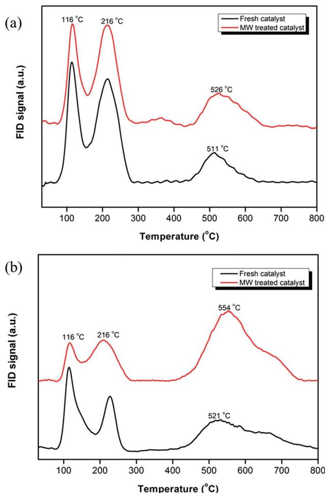
Fig. 6 TPSR profiles recorded from methanation studies using the (a) 0.7K/10Fe/SiO<sub>2</sub> and (b) 1.0K/10Fe/SiO<sub>2</sub> catalysts.
