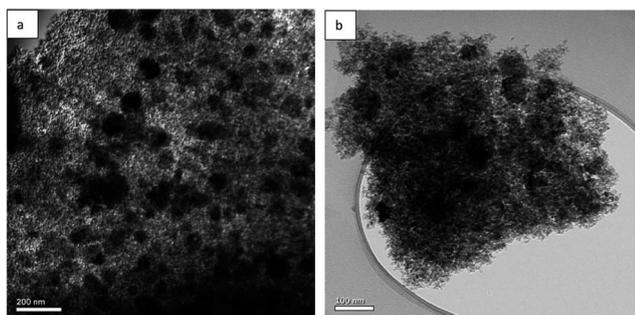
Fig. 1 TEM images of 0.2K/10Fe/SiO<sub>2</sub> and 0.7K/10Fe/SiO<sub>2</sub>.
