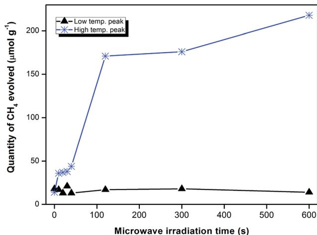
Fig. 4 Variation in the methane content produced by the low and high temperature TPSR peaks as a function of the microwave irradiation time. Data shown is for the 1.0K/10Fe/SiO<sub>2</sub> catalyst.
