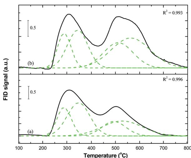
**Fig. 2** TPSR profiles of 0.2K/10Fe/SiO<sub>2</sub> (unmodified) and 0.2K/10Fe/SiO<sub>2</sub>-MW (modified using microwave radiation) catalysts displaying the evolution of methane as a function of temperature. Data on the individual contributions of the carbon species are tabulated in Table 1.
