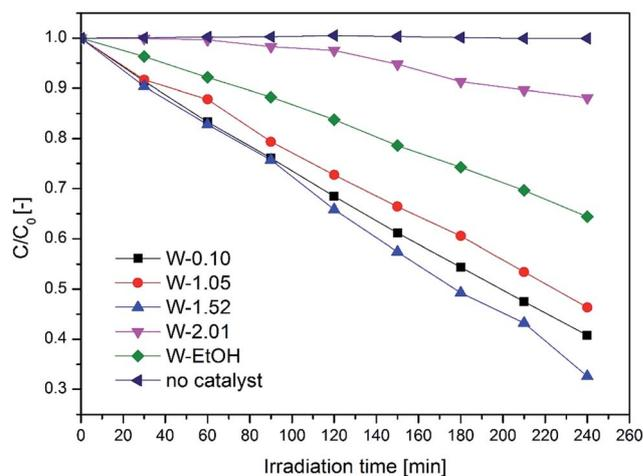
Fig. 10 Photocatalytic performance of the as-prepared WO<sub>3</sub> nanostructures.
