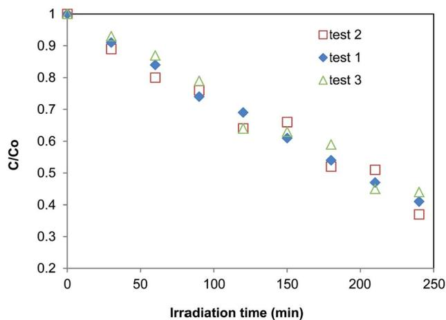
Fig. 11 Recycling tests of W-0.1 photocatalytic performance.
