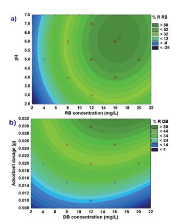
Fig. 4 Contour plots of combined effects of pH-RB concentration (a) and adsorbent dosage-DB concentration (b) on the % removal of RB and DB, respectively. The actual values of other factors are mean values (coded values 0).
