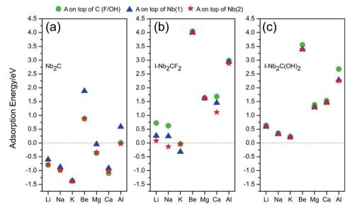
Adsorption energies for atom species A (A = Li, Na, K, Be, Mg, Ca, Al) on (a) Nb<sub>2</sub>C, (b)  $I-Nb_2CF_2$  and (c)  $I-Nb_2C(OH)_2$  at different adsorption Fia. 3 sites
