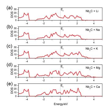
Fig. 5  $\,$  Total DOS of the bare  $\,$ Nb $_2$ C monolayer after (a) Li, (b) Na, (c) K, (d) Mg and (e) Ca adsorption. The dotted vertical lines denote the Fermi levels.
