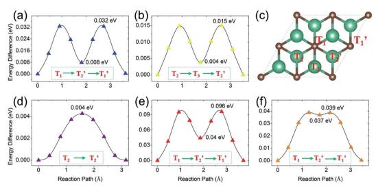
Fig. 6 The diffusion barrier profiles of (a) Li, (b) Na, (d) K, (e) Mg and (f) Ca on the Nb<sub>2</sub>C monolayer. The migration paths for A' diffusion are shown in the inset of each panel. (c) labelling of the high symmetry points appearing in the diffusion paths.  $T_1$  and  $T_1$  represent the two sites on top of two neighboring C atoms.  $T_2$  and  $T_2$  represent the two sites on top of two neighboring Nb(2) atoms.  $T_3$  represents the site on top of the Nb(1) atom.
