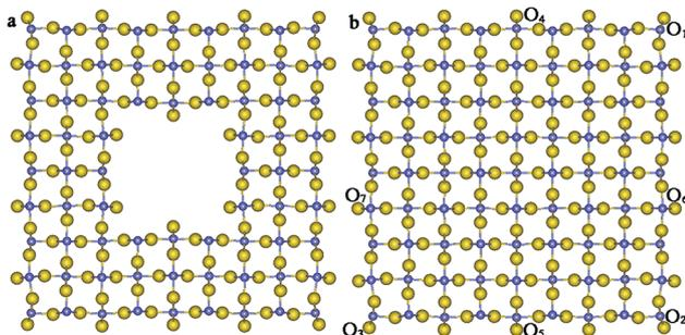
Fig. 2 Cross-sectional images of the nanostructures of rutile morphology: (a) FNT with 72 formula units per UC and (b) largest FNW with 81 formula units per UC.  $O_1$ ,  $O_2$ ,  $O_3$  are corner oxygen atoms;  $O_4$ ,  $O_5$ ,  $O_6$  and  $O_7$  are edge oxygen atoms.
