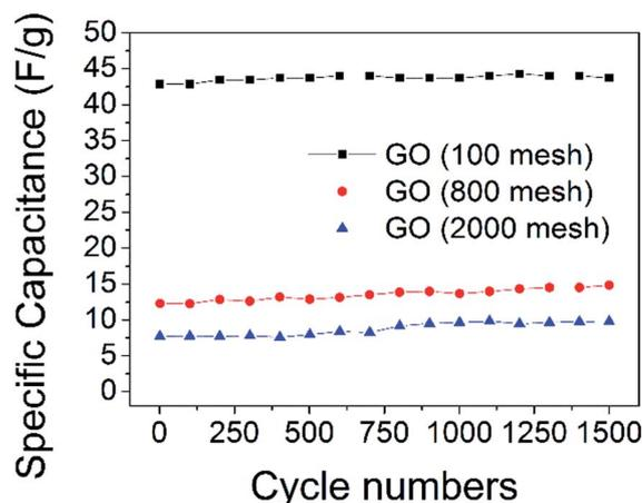
Fig. 9 Specific capacitance of the GO electrodes for 1500 cycles, charge–discharge tests at a current density of 1 A g<sup>-1</sup>.
