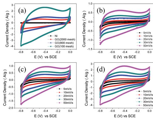
Fig. 6 (a) Cyclic voltammograms of different electrode materials at 50 mV s<sup>-1</sup>. Cyclic voltammograms at different voltage scanning rates of (b) GO (2000 mesh), (c) GO (800 mesh), and (d) GO (100 mesh).
