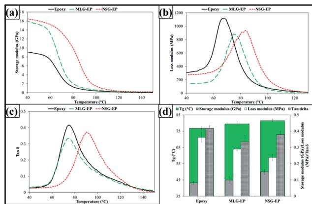
Fig. 5 Dynamic mechanical properties: (a) storage modulus, (b) loss modulus, (c)  $\tan \delta$ , and (d)  $T_g$ , and values of storage modulus, loss modulus and  $\tan \delta$  at  $T_g$ .
