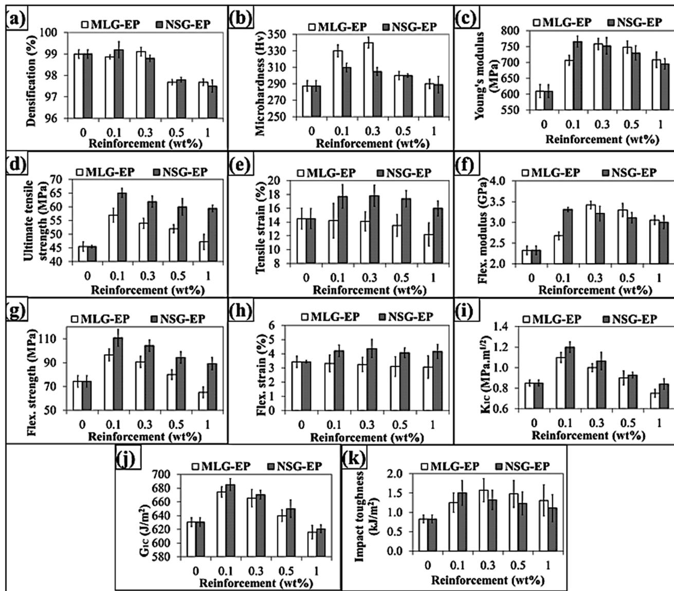
Fig. 4 Densification and mechanical properties: (a) densification, (b) microhardness (Hv), (c) Young's modulus, (d) ultimate tensile strength, (e) tensile strain (%), (f) flexural modulus, (g) flexural strength, (h) flexural strain (%), (i)  $K_{1C}$ , (j)  $G_{1C}$ , and (k) Charpy impact toughness.
