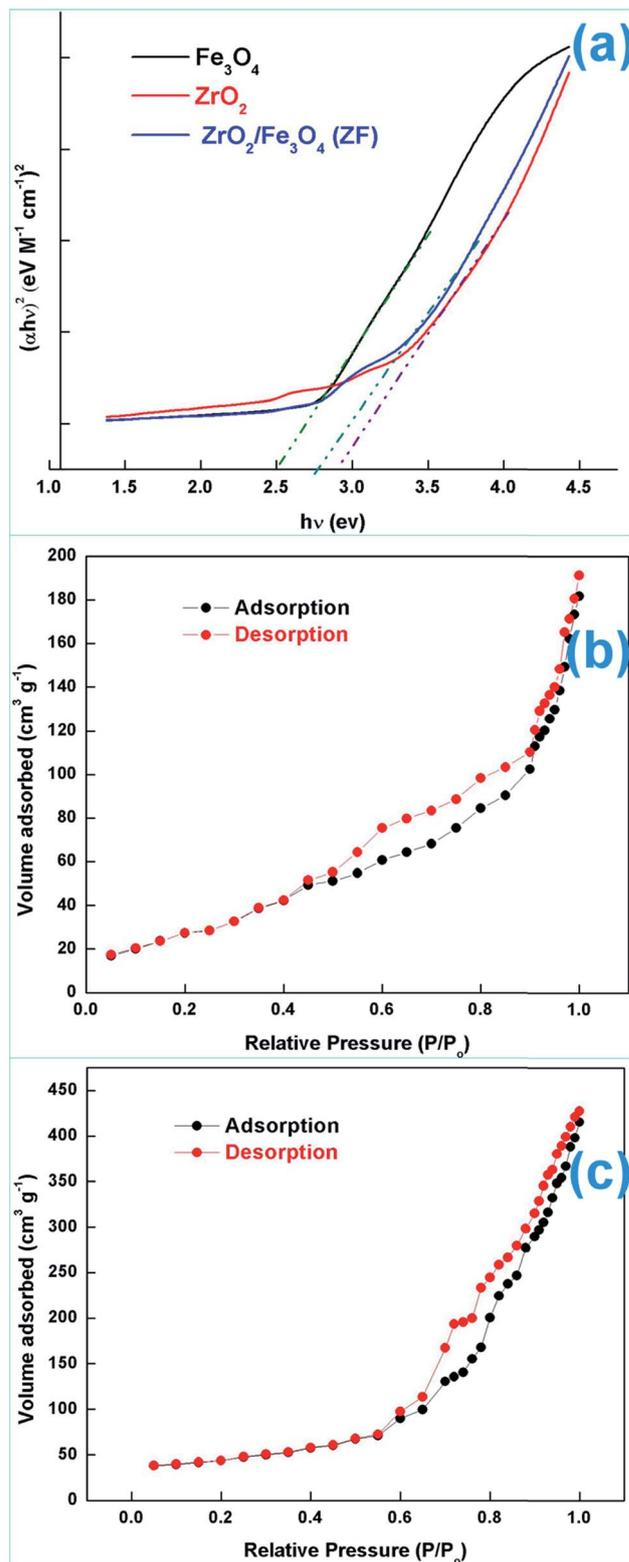
Fig. 5 (a) Tauc plots, (b) N<sub>2</sub> adsorption–desorption isotherms for ZF and (c) N<sub>2</sub> adsorption–desorption isotherms for ZFC.
