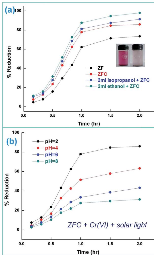
Fig. 7 (a) Photoreduction of Cr(vi) under solar light [initial pH 2], Cr(vi) = 70 mg L<sup>-1</sup> [temperature = 30 ± 0.5 °C] and (b) ZFC performance as photocatalyst with pH variation under solar light.
