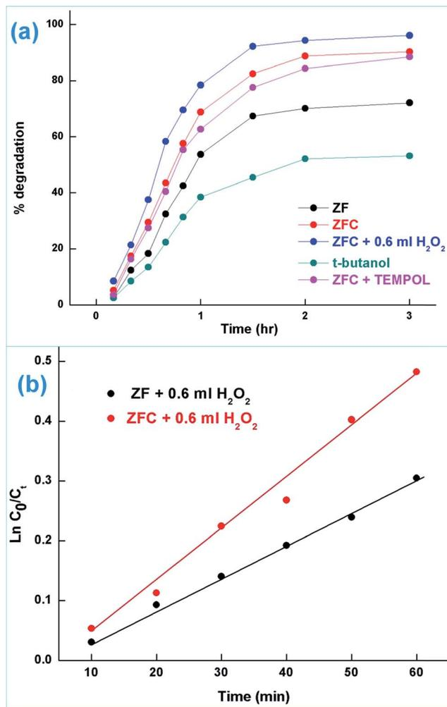
Fig. 8 (a) Degradation of 4-CP under solar light and (b) kinetics plots for 4-CP degradation by ZF and ZFC in the presence of H<sub>2</sub>O<sub>2</sub> under solar light (initial pH = 5.5, initial conc. of 4-CP = 20 mg L<sup>-1</sup>, and temperature = 30 ± 0.5 °C).
