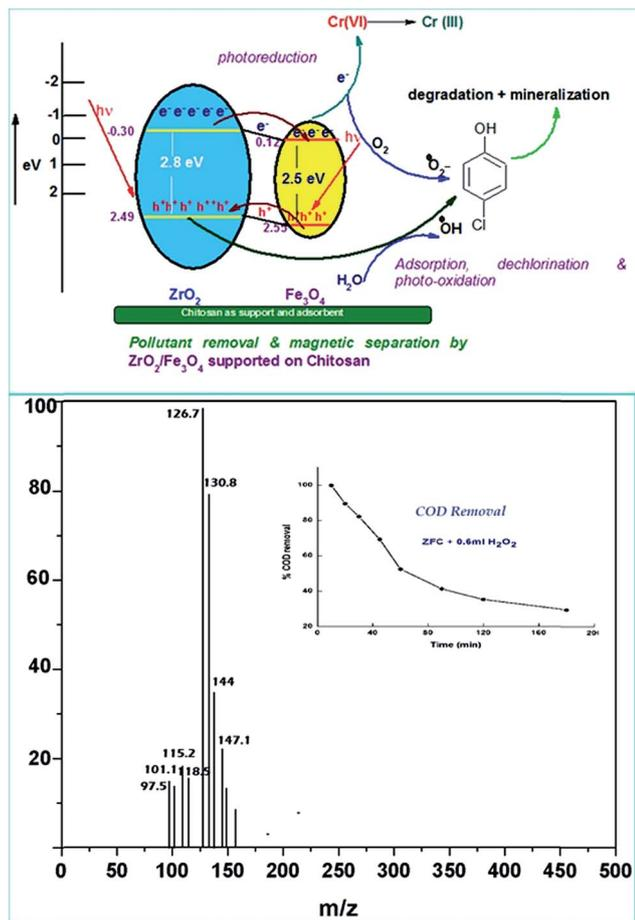
Fig. 9 (a) Band gap structure for the  $\text{ZrO}_2\text{-Fe}_3\text{O}_4$  heterostructure and mechanism of  $\text{Cr}(\text{vi})$  reduction and 4-CP removal and (b) mass spectrum of the solution containing 4-CP after 1 hour of degradation under solar light in the presence of ZFC (inset: COD removal in the presence of ZFC).
