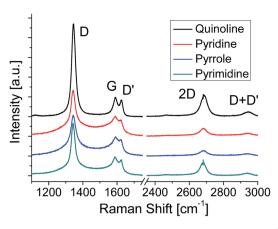
Fig. 3 Raman spectra of N-doped graphenes synthesized at 500 °C.
