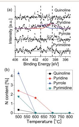
Fig. 5 (a) XPS N 1s spectra of the graphenes synthesized at  $600\,^{\circ}$ C. (b) Nitrogen content as a function of growth temperature for each of the source molecules.
