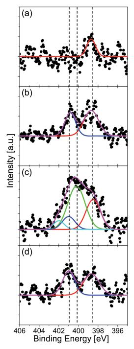
Fig. 4 XPS N 1s spectra of N-doped graphenes synthesized at  $500\,^{\circ}$ C from (a) quinoline, (b) pyridine, (c) pyrrole, and (d) pyrimidine. Each spectrum is fitted with three Gaussian functions: pyridinic- (red line), pyrrolic- (green line), and graphitic-N (blue line).
