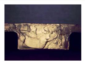
Fig. 3 Mirror housing exhibit stress cracking failure after liquid medium exposure.<sup>22</sup>
