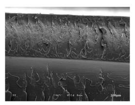
Fig. 5  $\,$  SEM image of intersecting network of cracks on the headlight lens.  $^{\rm 22}$
