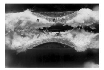
Fig. 13 Fractograph of stress corrosion crack growth of surface crack: ((I) starter notch; (II) stress corrosion crack growth; and (III) cracking in air brush like region). 469
