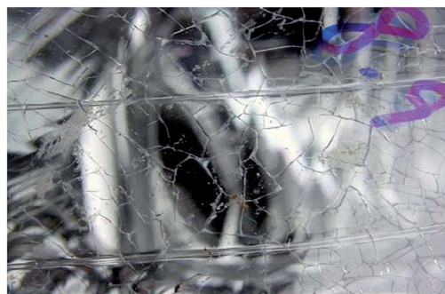
Fig. 4 Liquid medium effect on the headlight lens. 22
