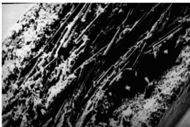
Fig. 8 Broken section of glass/polyester composite after 21 day immersion in water.<sup>14</sup>
