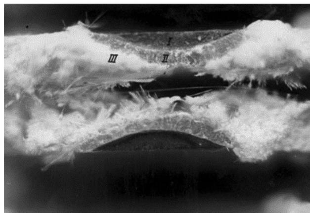
Fig. 13 Fractograph of stress corrosion crack growth of surface crack: (I) starter notch; (II) stress corrosion crack growth; and (III) cracking in air brush like region.<sup>169</sup>
