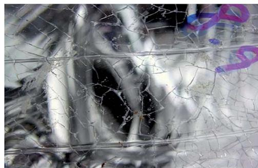
Fig. 4 Liquid medium effect on the headlight lens.<sup>22</sup>
