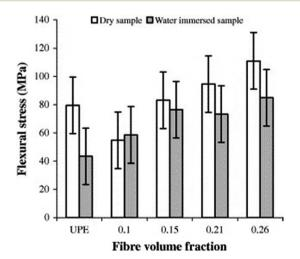
Fig. 10 The flexural stress of hemp fibre reinforced unsaturated polyester.<sup>98</sup>
