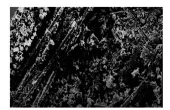
Fig. 7 Broken section of glass/polyester composite sample without water exposure.<sup>14</sup>
