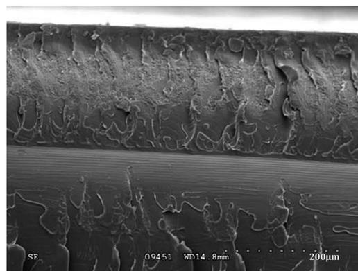
Fig. 5 SEM image of intersecting network of cracks on the headlight lens.<sup>22</sup>
