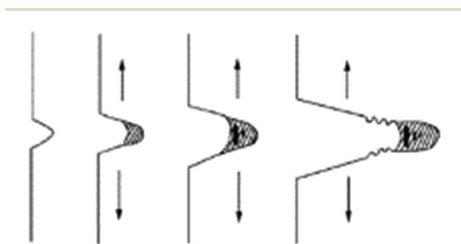
Fig. 11 Crack developments under ESC condition.<sup>155</sup>
