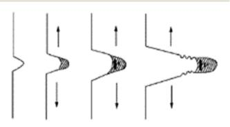
Fig. 11 Crack developments under ESC condition. 155
