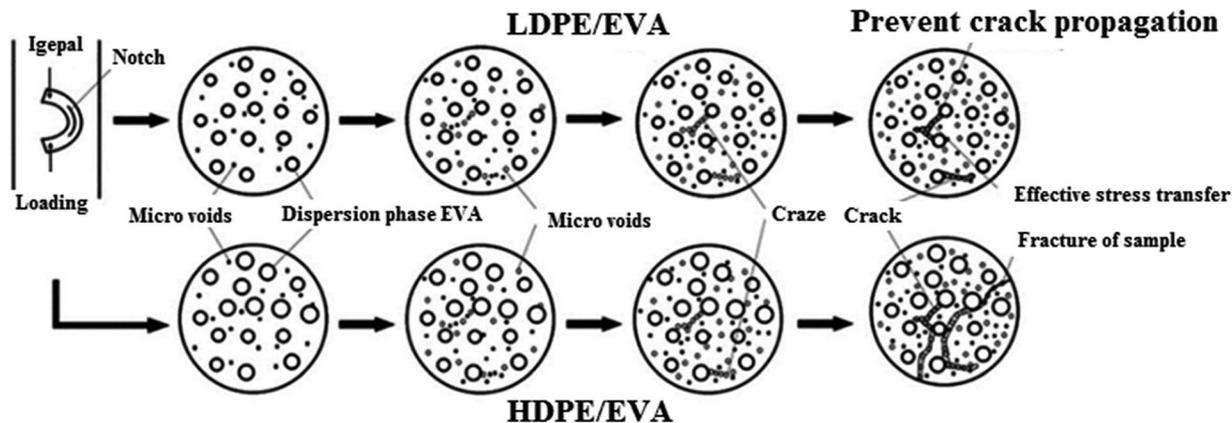
Fig. 12 The failure mechanisms of LDPE/EVA and HDPE/EVA blends.<sup>191</sup>
