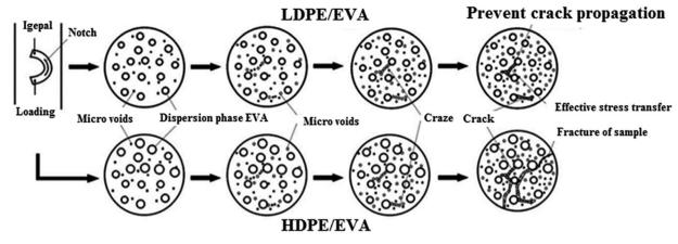
Fig. 12 The failure mechanisms of LDPE/EVA and HDPE/EVA blends. 191
