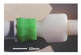
Fig. 2 Macrograph of brittle cracks from gate in male luer of connector.<sup>31</sup>
