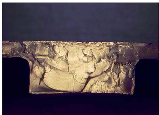
Fig. 3 Mirror housing exhibit stress cracking failure after liquid medium exposure.<sup>22</sup>
