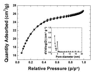
Fig. 2  $\,{\rm N_2}$  adsorption/desorption isotherms of APC material, inset show pore size distribution.
