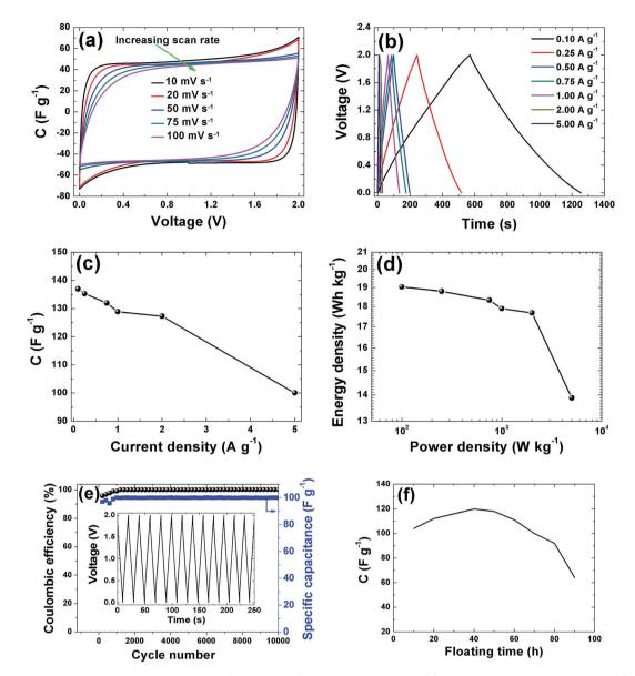
Fig. 7 Electrochemical performances tests for the APC in  $1 \text{ M Na}_2\text{SO}_4$  aqueous electrolyte: (a) CV curves at different scan rates, (b) CD curves at different current densities, (c) dependence of specific capacitance on current density, (d) Ragone plot (e) coulombic efficiency and gravimetric capacitance vs. cycle number and (f) 100 h voltage holding vs. capacitance.
