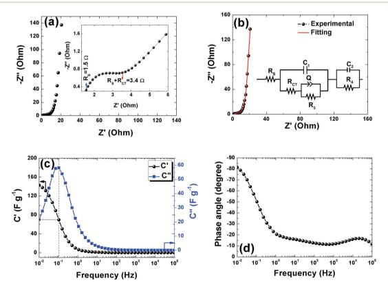
Fig. 8 (a) and (b) Nyquist plots for the APC based cell in  $1 \text{ M Na}_2\text{SO}_4$  with magnifications of the high to mid frequency region shown in the inset and fitted with equivalent circuit shown in the inset respectively, (c) the real and imaginary part of the cell gravimetric capacitance vs. frequency (black and blue curves) (d) Bode plot for the phase angle vs. frequency.
