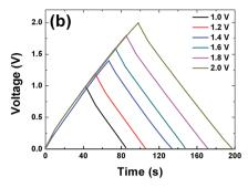
Fig. 6 (a) Cyclic voltammogram at 20 mV s<sup>-1</sup> and (b) galvanostatic charge–discharge at profiles of the APC at 0.5 A g<sup>-1</sup> at different voltage ranges respectively.
