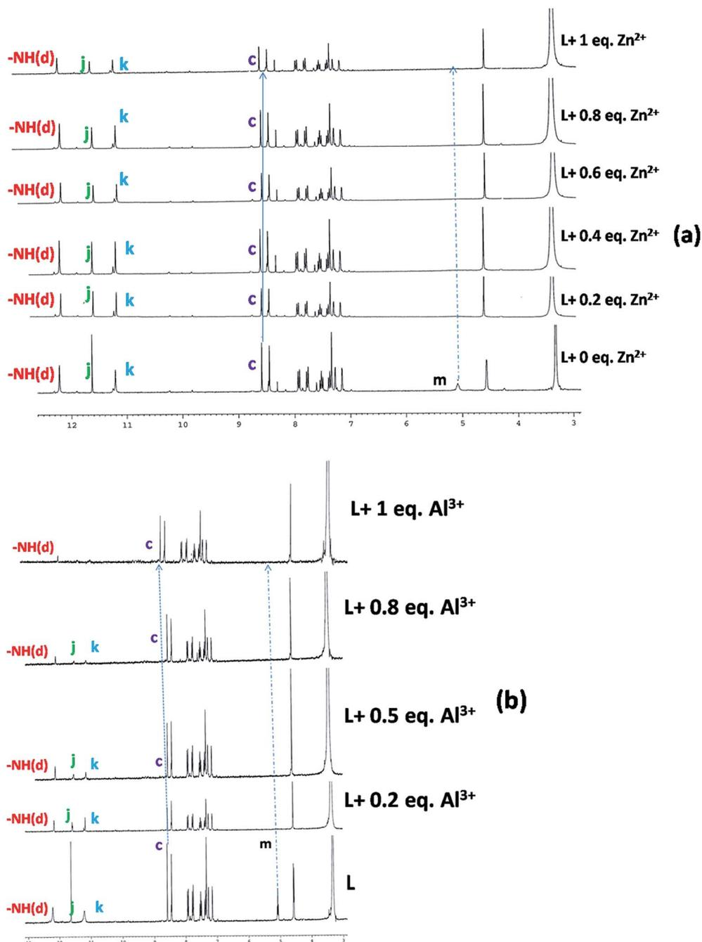
Fig. 6  $^1\text{H-NMR}$  titration of the free ligand ( $\text{L} = \text{H}_3\text{SAL-NH}$ ) and with the addition of 1 equivalent of  $\text{Zn}^{2+}$  (a) and  $\text{Al}^{3+}$  (b) in  $\text{DMSO-d}_6$  recorded on a 300 MHz Bruker NMR spectrometer.
