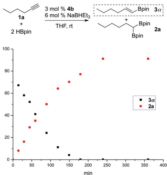
**Fig. 1** Profile of sequential hydroboration of 1-hexyne (**1a**) with 2 equiv. of HBpin catalyzed by 3 mol% **4b** and 6 mol% NaBHET<sub>3</sub> in THF at room temperature.
