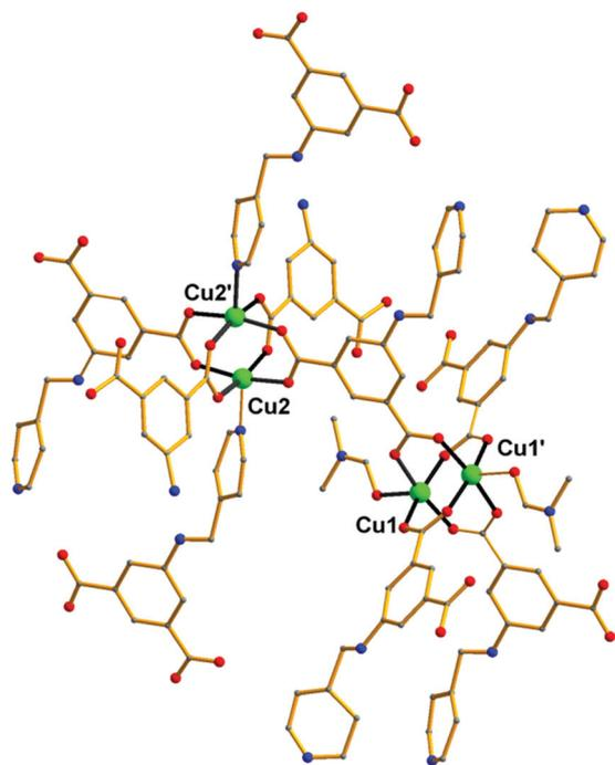
**Fig. 1** Representation of the connectivity of the  $[\text{Cu}_2^{2+}]_2$  paddle wheel SBUs through the  $\text{PEIP}^{2-}$  ligand in **Cu-PEIP**. Colour code: Cu green, O red, N blue, C gray. H atoms are omitted for clarity.
