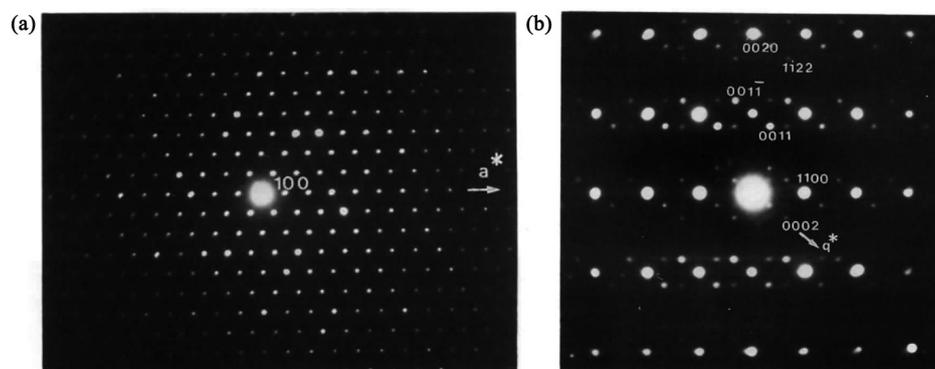
**Fig. 10** Electron diffraction pattern of  $\text{Ba}_{0.85}\text{Ca}_{2.15}\text{In}_6\text{O}_{12}$ . (a) [001] zone axis. (b) [100] zone axis showing extra spots appearing near the main spots of the hexagonal lattice. Reproduced with permission of the International Union of Crystallography from ref. 103.
