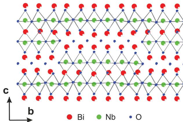
**Fig. 13** Part of the structure of  $\text{Bi}_5\text{Nb}_3\text{O}_{15}$  showing both the continuous and discontinuous perovskite blocks and  $[\text{Bi}_2\text{O}_2]$  slabs. Reproduced with permission from ref. 115. Copyright 2013 American Chemical Society.
