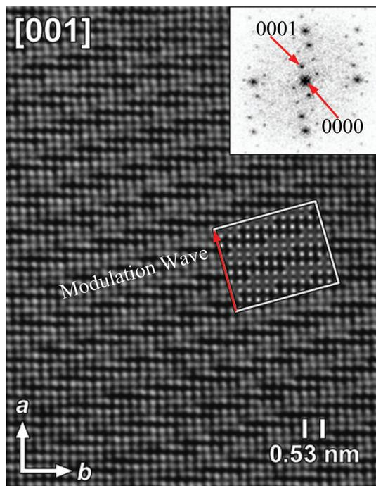
**Fig. 3** [001] HRTEM image and the corresponding FT pattern of the incommensurately modulated  $\text{KNd}(\text{MoO}_4)_2$ . The inset represents a calculated image based on the model, for a focus value of  $-60$  nm and a thickness of  $2$  nm. Reproduced with permission from ref. 23. Copyright 2006 American Chemical Society.
