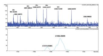
Fig. 5 ESI-MS of His3 Mn<sup>III</sup>Mb after reacting with 20 equiv. KHSO<sub>5</sub> for
