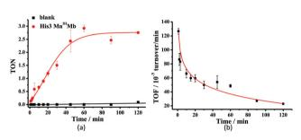
Fig. 6 Time course plots of (a) turnover number (TON) with or without His3 Mn<sup>III</sup>Mb, and (b) turnover frequency (TOF) of styrene epoxidation catalyzed by His3 Mn<sup>III</sup>Mb. TON and TOF were calculated based on the amount of styrene. The initial TOF was calculated at 1 min.
