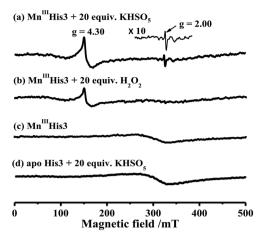
Fig. 4 X-band EPR spectra of (a) 1.0 mM His3 Mn<sup>III</sup>Mb in 50 mM PBS buffer (pH 7.4), and (b) in the presence of 20 equiv. H<sub>2</sub>O<sub>2</sub> or (c) 20 equiv. KHSO<sub>5</sub>, and (d) apo-His3 Mb in the presence of 20 equiv. KHSO<sub>5</sub>. The EPR spectra are recorded at -170 °C.
