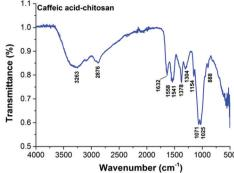
Fig. 3 FT-IR spectra of chitosan and chitosan-caffeic acid.
