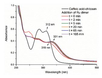
**Fig. 5** The UV-vis spectra for the reaction of Ru dimer with caffeic acid-modified chitosan at different reaction times, [Ru dimer] =  $2.0 \times 10^{-5}$  mol L<sup>-1</sup>, [caffeic acid in caffeic acid-modified chitosan] =  $4.0 \times 10^{-5}$  mol L<sup>-1</sup>, in water.
