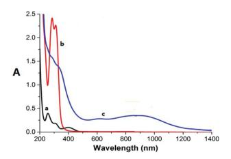
Fig. 4 The UV-vis spectra of Ru dimer (a), caffeic acid-modified chitosan (b) and Ru-caffeic acid-modified chitosan (c), [Ru dimer] =  $1.5 \times 10^{-4}$  mol L<sup>-1</sup>, [caffeic acid-chitosan] = 0.4 mg mL<sup>-1</sup>, in water.
