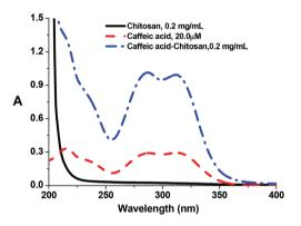
Fig. 1 UV spectra of chitosan (0.2 mg mL<sup>-1</sup>), caffeic acid (20 µM), chitosan-caffeic acid (0.2 mg mL<sup>-1</sup>) in 18 m $\Omega$  cm water, T = 298 K.
