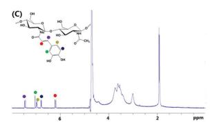
Fig. 2 <sup>1</sup>H NMR spectra of (A) chitosan in 1% CD<sub>3</sub>COOD in D<sub>2</sub>O, (B) caffeic acid in CD<sub>3</sub>OD, and (C) chitosan-caffeic acid in D<sub>2</sub>O.
