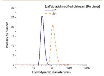
Fig. 7 Dynamic light scattering of Ru-caffeic acid modified chitosan at two different ratios. Spectra were recorded at 25 °C; 2 mg mL<sup>-1</sup>; the solutions were not filtered before analysis.
