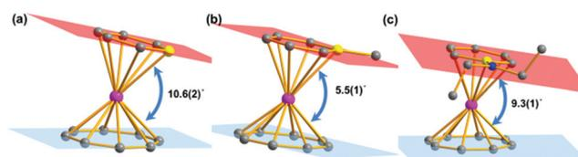
Fig. 1 Molecular structures of **1Er–3Er**. (a), (b) and (c) Represent **1Er**, **2Er** and **3Er**, respectively. Color code: pink, Er, dark grey, C, yellow, B, blue, N. Hydrogen atoms are omitted for clarity.
