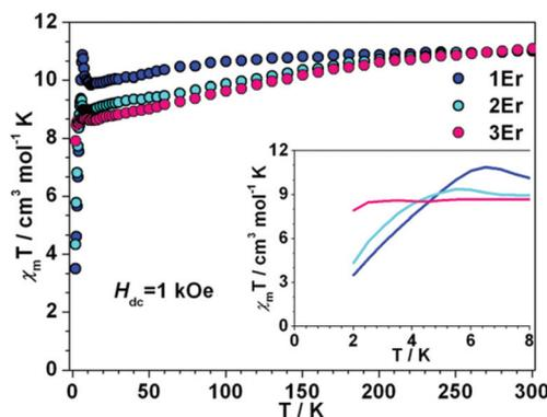
Fig. 2 Temperature dependence of the dc magnetic susceptibility time temperature  $\chi_m T$  for **1Er–3Er** under 1 kOe applied magnetic field. (Inset) Expanded view of  $\chi_m T$  vs.  $T$  plots below 8 K.
