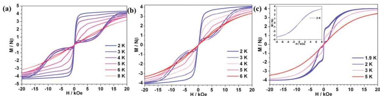
**Fig. 4** Variable-field magnetization data for **1Er** (a), **2Er** (b), **3Er** (c inset) and diluted **3Er** (c) were collected at the average field sweeping rate of  $1.9 \text{ mT s}^{-1}$ . As a result of the QTM, the coercive field was not observed.
