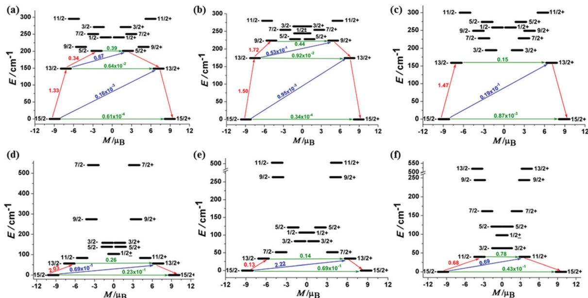
Fig. 5 The magnetization blocking barriers in complexes **1Er**–**6Dy**, represented by (a)–(f). The thick black lines represent Kramer's doublets as a function of their magnetic moment along the magnetic axis. The green lines correspond to diagonal quantum tunneling of magnetization (QTM), the blue lines represent the off-diagonal relaxation process. The numbers at each arrow stand for the mean absolute value of the corresponding matrix element of the transition magnetic moment.
